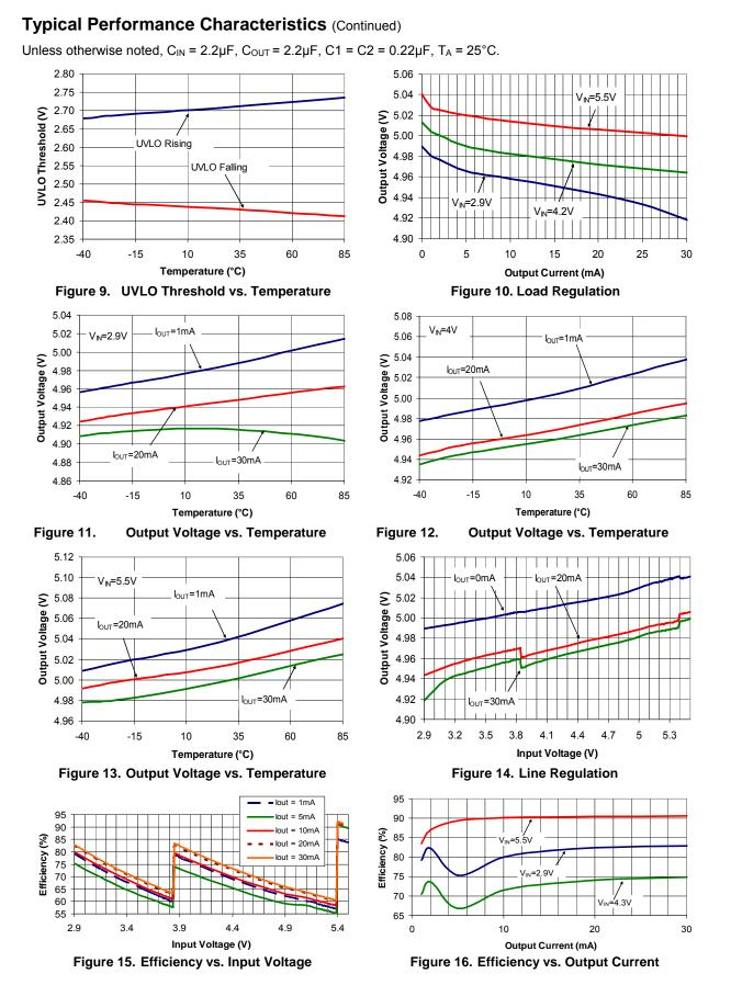
FAN5665 — High-Efficiency, Adaptive Charge Pump 5V Boost
