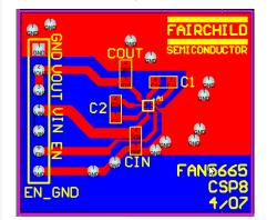
Figure 42. PCB Layout
