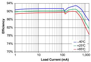
Figure 5. Efficiency vs. Load Current and Temperature,  $V_{\text{IN}}$  = 3.6 V ,  $V_{\text{OUT}}$  = 1.8 V, Auto Mode
