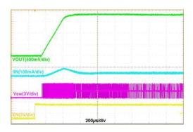
Figure 20. Start-up, V<sub>IN</sub>= 3.6 V, V<sub>OUT</sub>= 1.8 V, 50 mA Resistive Load, Auto Mode
