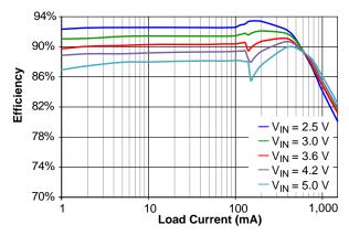
Figure 4. Efficiency vs. Load Current and Input Voltage, V<sub>OUT</sub> = 1.8 V, Auto Mode
