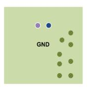
Layer 2 should be a solid ground layer, to shield VOUT from capacitive coupling of the fast edges of SW node.
