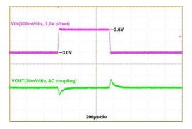
Figure 19. Line Transient,  $V_{IN}$  = 3.0 V  $\leftrightarrow$  3.6 V,  $V_{OUT}$  = 1.8 V, 10  $\mu$ s Edge, 300 mA Load, Auto Mode
