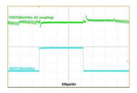
Figure 16. Load Transient,  $V_{IN}$  = 3.6 V,  $V_{OUT}$  = 1.8 V, 5 mA  $\leftrightarrow$ 300 mA, 1  $\mu s$  Edge, Auto Mode
