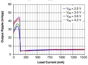
Figure 9. Output Ripple vs. Load Current and Input Voltage, V<sub>OUT</sub> = 1.8 V, Auto Mode
