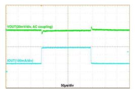
Figure 17. Load Transient,  $V_{IN}$  = 3.6 V,  $V_{OUT}$  = 1.8 V, 100 mA  $\leftrightarrow$  300 mA, 1  $\mu$ s Edge, Auto Mode
