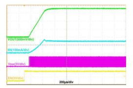
Figure 21. Start-up, V<sub>IN</sub>= 3.6 V, V<sub>OUT</sub>= 1.8 V, 300 mA Resistive Load, Auto Mode
