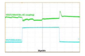
Figure 18. Load Transient,  $V_{IN}$  = 3.6 V,  $V_{OUT}$  = 1.8 V, 10 mA  $\leftrightarrow$ 1500 mA, 1  $\mu s$  Edge, Auto Mode
