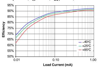
Figure 7. Efficiency vs. Load Current and Temperature,  $V_{\text{IN}}$  = 3.6 V ,  $V_{\text{OUT}}$  = 1.8 V, SLIQ Mode
