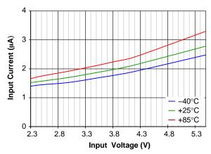
Figure 12. Quiescent Current vs. Input Voltage and Temperature, VOUT = 1.8 V, Auto Mode
