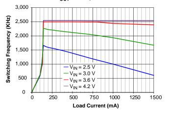
Figure 8. Frequency vs. Load Current and Input Voltage, Auto Mode, V<sub>OUT</sub> = 1.8 V, Auto Mode
