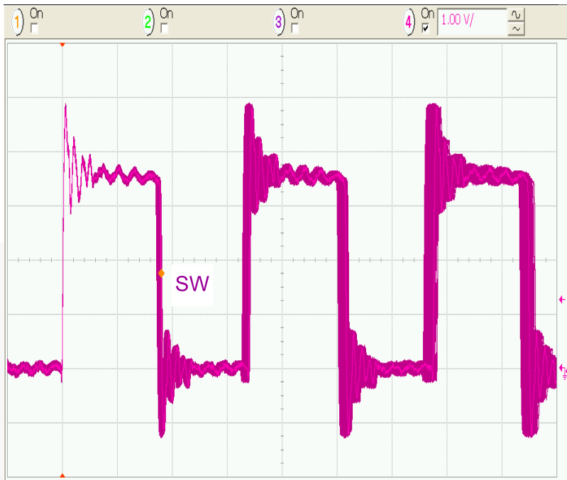
Figure 39. SW-Node Jitter (Infinite Persistence), I_{LOAD} = 200mA , 50ns/div.
