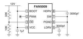
Figure 2. Test Circuit
