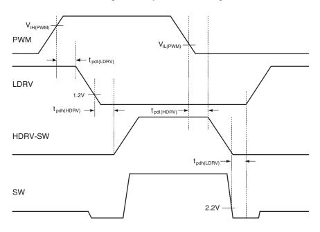
Figure 4. Adaptive Gate Drive Timing
