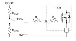
Figure 5. Driver dissipation model
