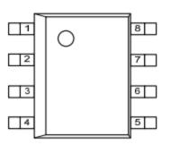
Figure 2. Pin Assignment (Top View)
