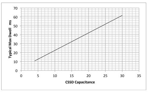
Figure 5: T<sub>DMAX</sub> as function of external CSSD capacitor
