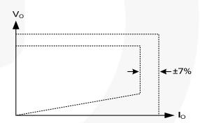
Figure 1. Typical Output V-I Characteristic
