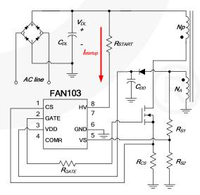
Figure 25. HV Startup Circuit
