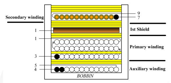
Figure 29. Bobbin Winding Diagram
