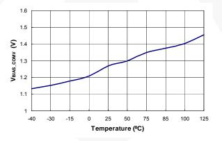
Figure 19. Output Clamp Voltage ( $V_{\text{CLAMP}}$ ) vs. Temperature
