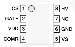
Figure 5. Pin Configuration
