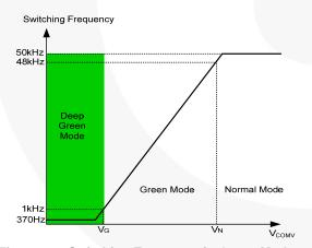
Figure 23. Switching Frequency in Green Mode
