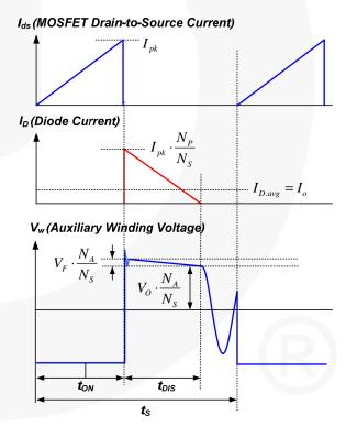
Figure 22. Key Waveforms of DCM Flyback Converter
