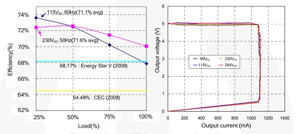
Figure 27. Measured Efficiency and Output Regulation
