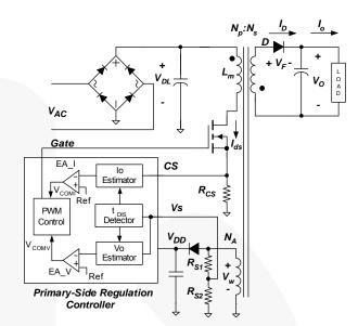
Figure 21. Simplified PSR Flyback Converter Circuit
