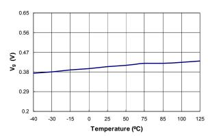
Figure 16. Green Mode Starting Voltage on EA\_V  $(V_N)$  vs. Temperature
