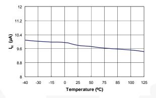
Figure 18. IC Bias Current (Itc) vs. Temperature
