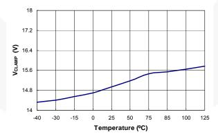
Figure 20. Variation Test Voltage on COMR Pin for Cable Compensation (V<sub>COMR</sub>) vs. Temperature
