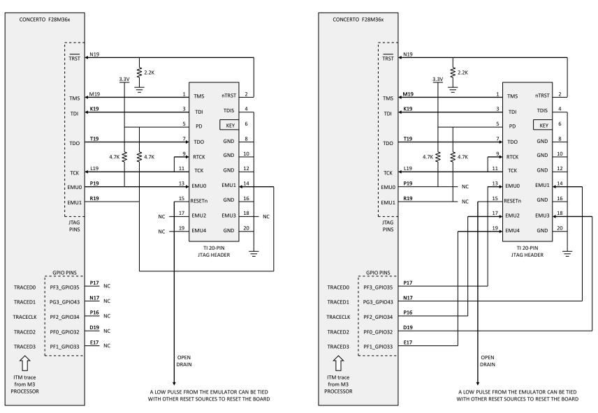
Figure 2-18. Connecting to TI 20-Pin JTAG Emulator Header
