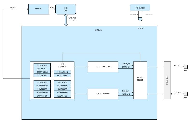
Figure 6-11. I2C (Cortex™-M3)
