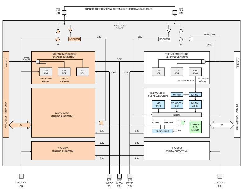
Figure 2-6. Voltage Regulation and Monitoring
