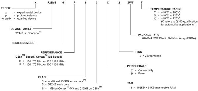
A. The additional 256KB is added to the Cortex™-M3 core (Connectivity Devices) or to the C28x™ core (Base Devices).
