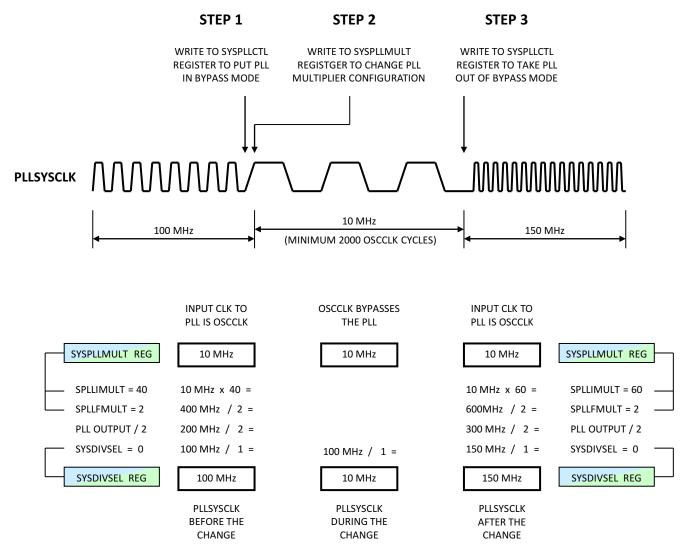
Figure 5-4. Changing the Frequency of the Main PLL
