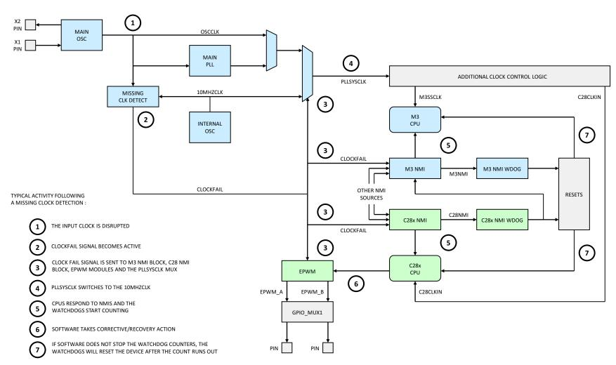
Figure 2-12. Missing Clock Detection
