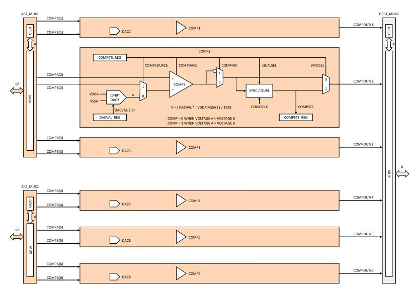
Figure 6-2. Comparator + DAC Units
