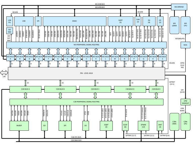
Figure 2-14. GPIO\_MUX1 Block
