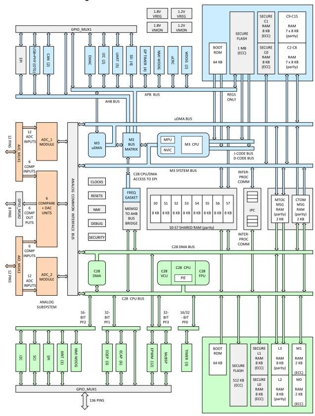
Figure 1-1. Functional Block Diagram
