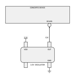
Figure 2-7. Connecting Input Clocks to a Concerto Device
