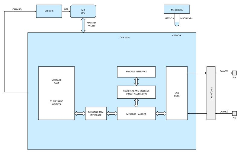
Figure 6-12. CAN (Cortex™-M3)
