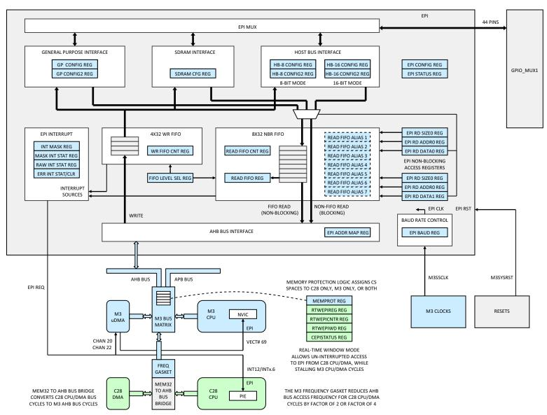
Figure 6-4. External Peripheral Interface (EPI)
