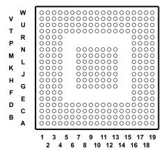
Figure 3-1. 289-Ball ZWT Ball Grid Array (Bottom View)
