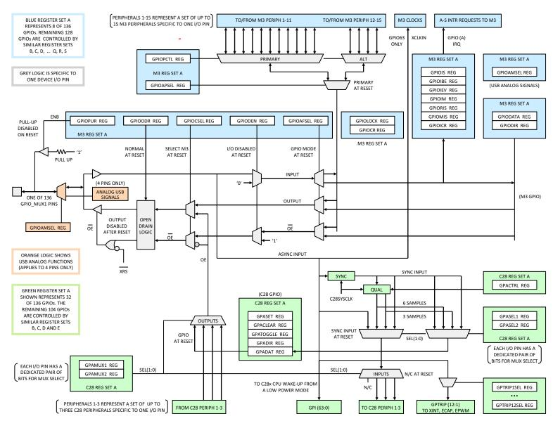
Figure 2-15. GPIO\_MUX1 Pin Mapping Through Register Set A
