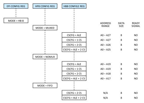
Figure 6-7. EPI 8-Bit Host Bus Mode
