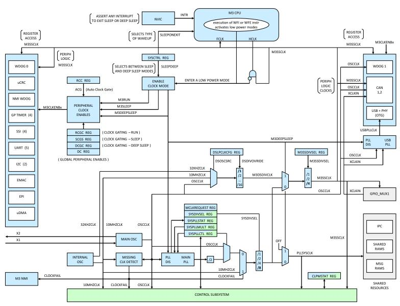
Figure 2-10. Cortex™-M3 Clocks and Low-Power Modes
