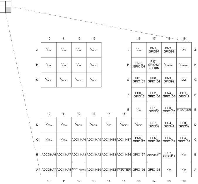
A. All I/Os, except for GPIO199, are glitch-free during power up and power down. See Section 2.11.
