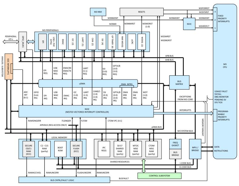
Figure 2-1. Master Subsystem
