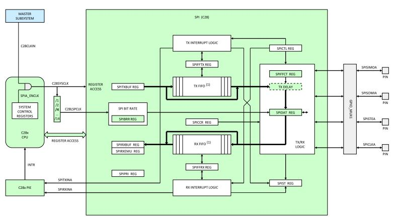
(1) RX FIFO AND TX FIFO CAN BE BYPASSED BY CONFIGURING BIT SPIFFENA OF THE SPIFFTX REGISTER
