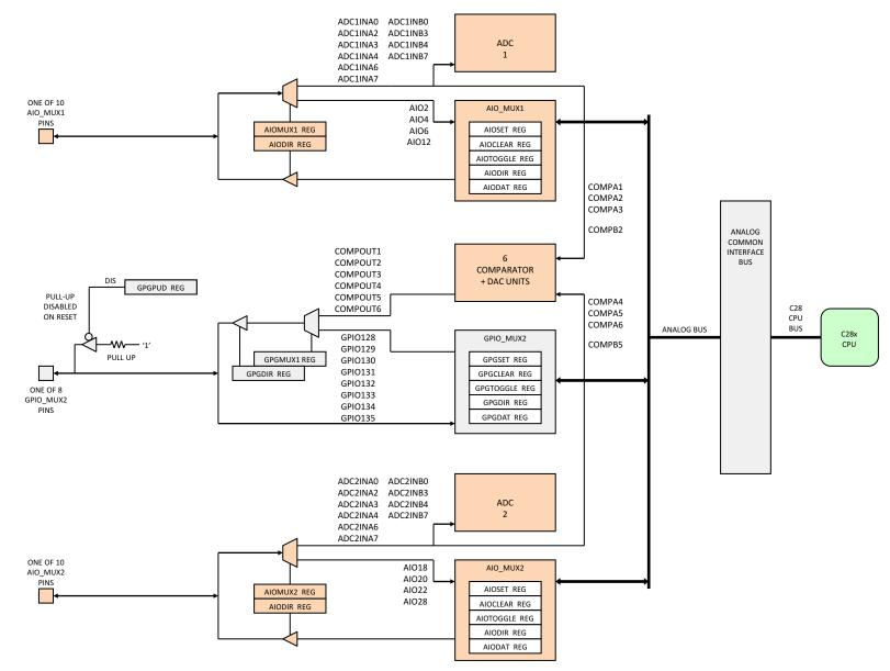
Figure 2-16. Pin Muxing on AIO\_MUX1, AIO\_MUX2, and GPIO\_MUX2
