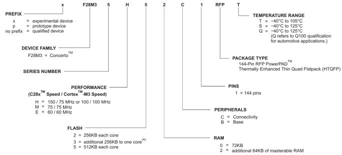
A. The additional 256KB is added to the Cortex<sup>™</sup>-M3 core (Connectivity Devices) or to the C28x<sup>™</sup> core (Base Devices).
