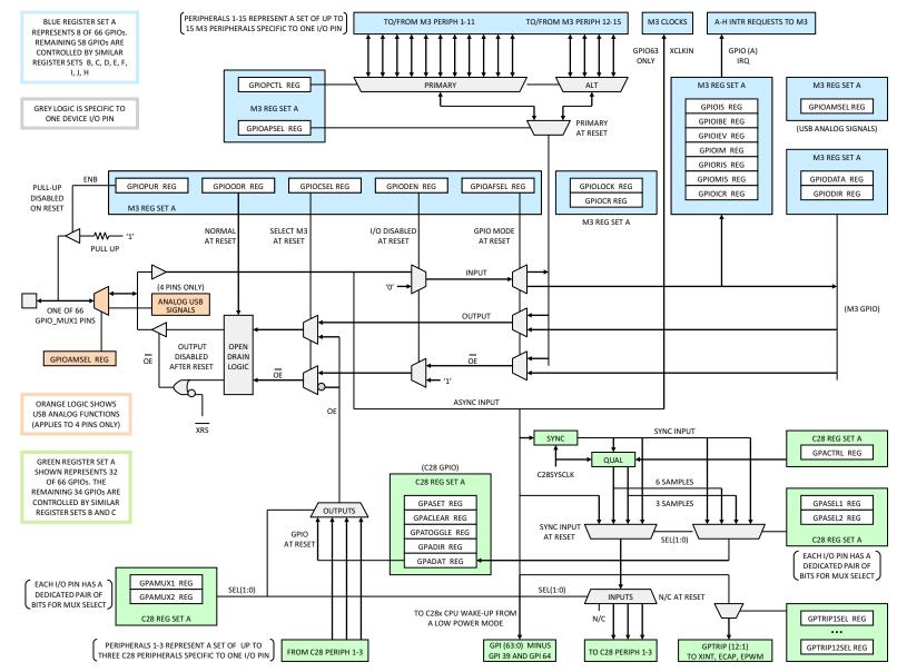
Figure 2-15. GPIO\_MUX1 Pin Mapping Through Register Set A
