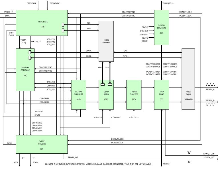
Figure 6-16. Internal Structure of PWM
