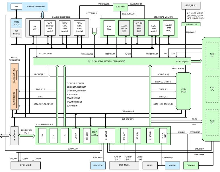
Figure 2-2. Control Subsystem
