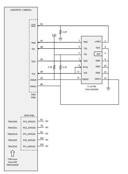
Figure 2-17. Connecting to TI 14-Pin JTAG Emulator Header
