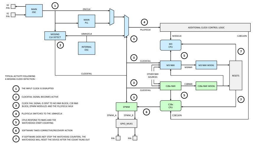
Figure 2-12. Missing Clock Detection
