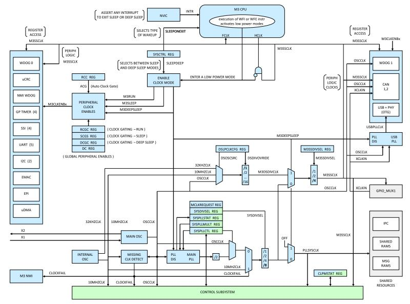
Figure 2-10. Cortex<sup>™</sup>-M3 Clocks and Low-Power Modes
