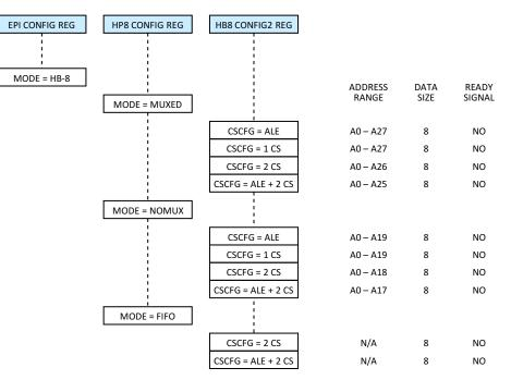
Figure 6-7. EPI 8-Bit Host Bus Mode
