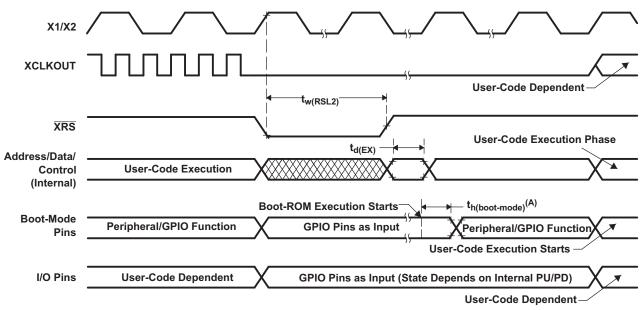
A. After reset, the Boot ROM code samples BOOT Mode pins. Based on the status of the Boot Mode pin, the boot code branches to destination memory or boot code function. If Boot ROM code executes after power-on conditions (in debugger environment), the Boot code execution time is based on the current M3SSCLK speed. The M3SSCLK will be based on user environment and could be with or without PLL enabled.
