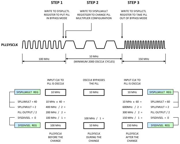
Figure 5-4. Changing the Frequency of the Main PLL
