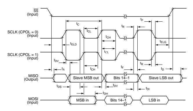
Figure 24. SPI Slave Timing (CPHA = 1)
