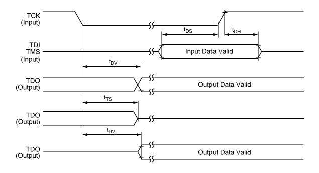
Figure 32. Test Access Port Timing Diagram
