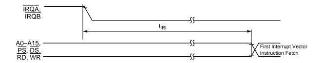
Figure 17. Interrupt from Wait State Timing
