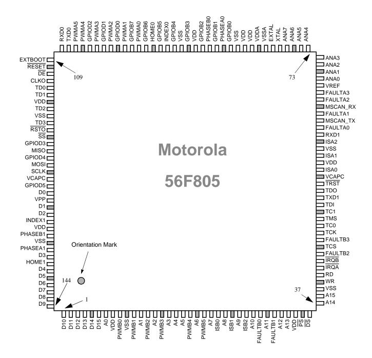
Figure 35. Top View, 56F805 144-pin LQFP Package
