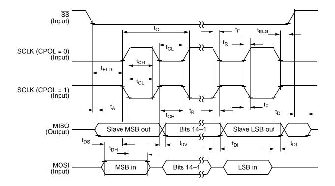
Figure 23. SPI Slave Timing (CPHA = 0)
