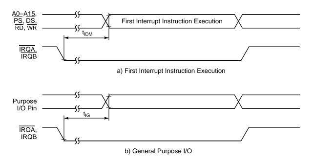
Figure 16. External Level-Sensitive Interrupt Timing
