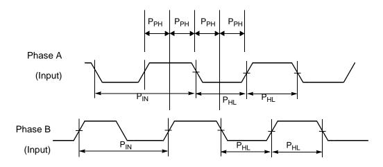
Figure 26. Quadrature Decoder Timing
