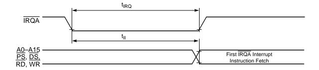
Figure 19. Recovery from Stop State Using IRQA Interrupt Service
