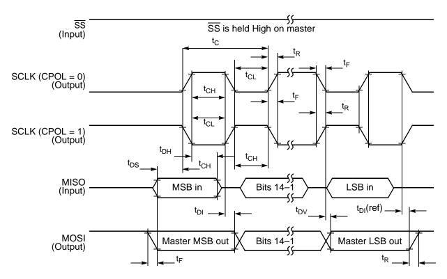
Figure 21. SPI Master Timing (CPHA = 0)
