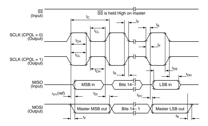
Figure 22. SPI Master Timing (CPHA = 1)
