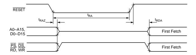
Figure 14. Asynchronous Reset Timing
