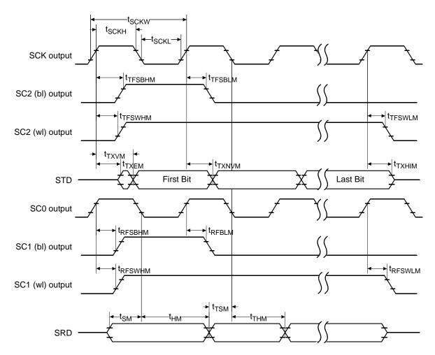
Figure 25. Master Mode Timing Diagram
