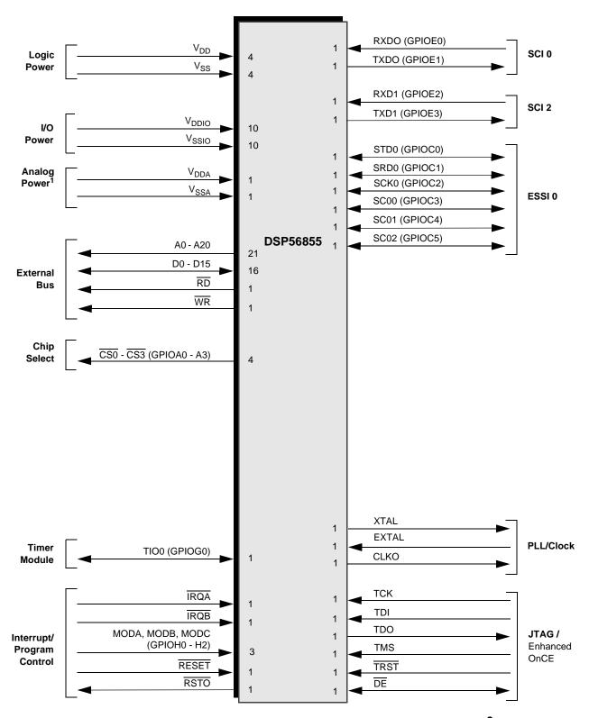
Figure 2. DSP56855 Signals Identified by Functional Group<sup>2</sup>
