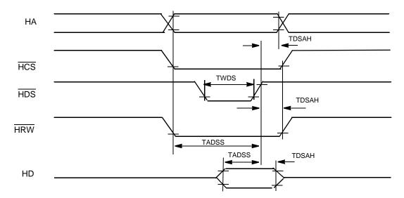
Figure 22. Single Strobe Write Mode
