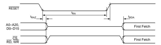
Figure 12. Asynchronous Reset Timing
