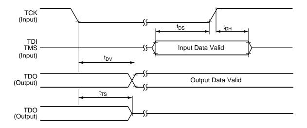
Figure 30. Test Access Port Timing Diagram
