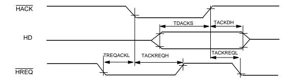
Figure 21. Host-to-DSP DMA Write Mode
