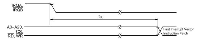
Figure 15. Interrupt from Wait State Timing
