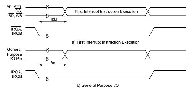
Figure 14. External Level-Sensitive Interrupt Timing
