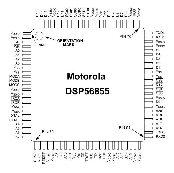
Figure 34. Top View, DSP56855 100-pin LQFP Package
