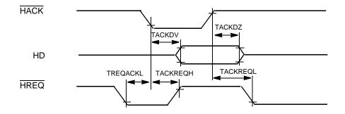
Figure 18. DSP-to-Host DMA Read Mode
