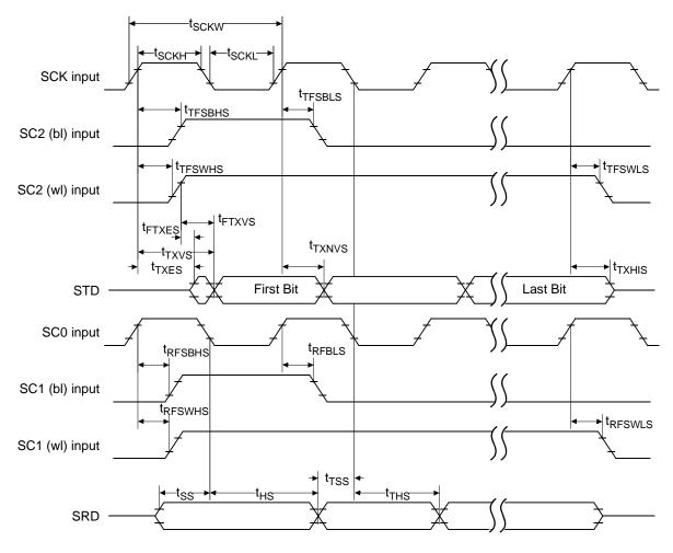
Figure 26. Slave Mode Clock Timing
