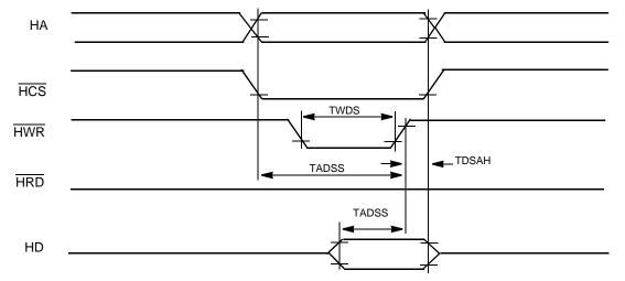
Figure 23. Dual Strobe Write Mode
