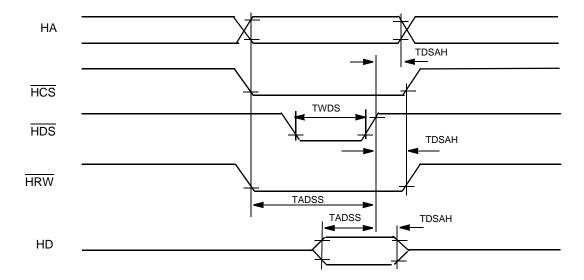
Figure 22. Single Strobe Write Mode
