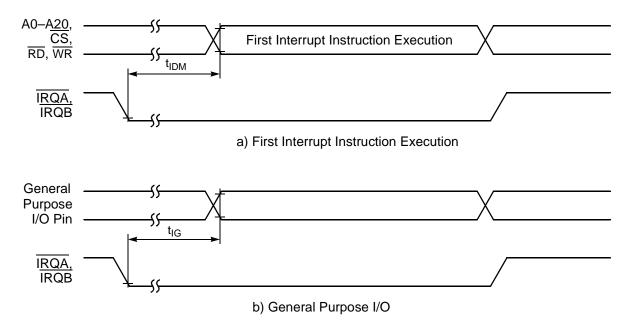
Figure 14. External Level-Sensitive Interrupt Timing
