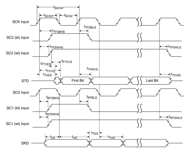
Figure 30. Slave Mode Clock Timing
