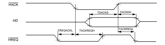
Figure 21. Host-to-DSP DMA Write Mode
