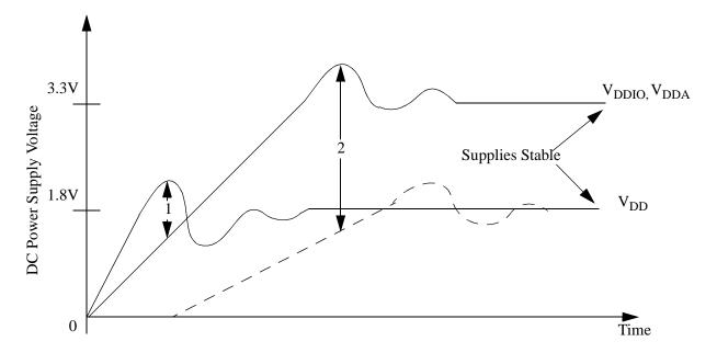
**Notes:** 1.  $V_{DD}$  rising before  $V_{DDIO}$ ,  $V_{DDA}$
