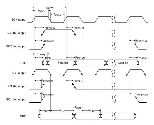
Figure 29. Master Mode Timing Diagram
