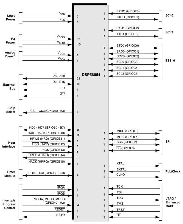
Figure 2. DSP56854 Signals Identified by Functional Group<sup>2</sup>
