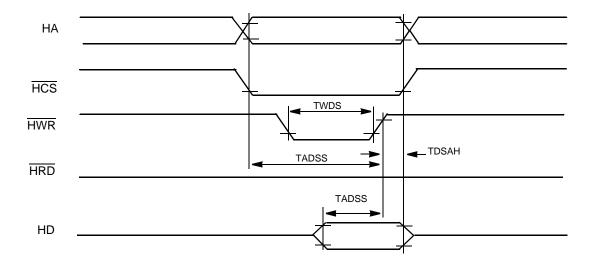
Figure 23. Dual Strobe Write Mode
