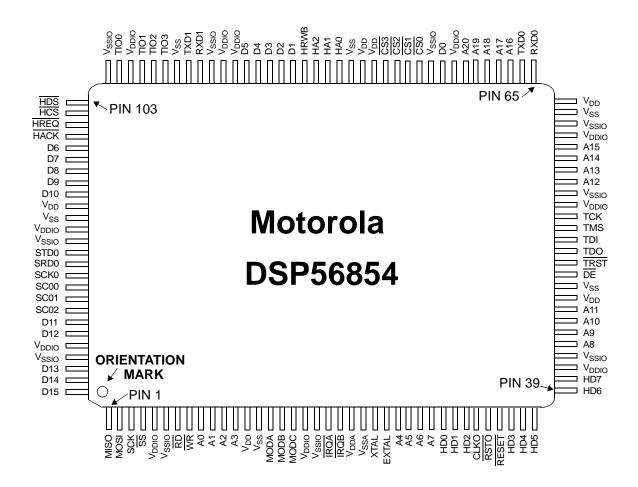
Figure 38. Top View, DSP56854 128-pin LQFP Package
