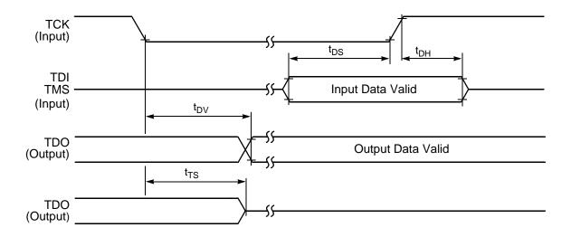
Figure 34. Test Access Port Timing Diagram
