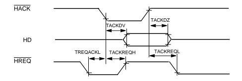
Figure 18. DSP-to-Host DMA Read Mode
