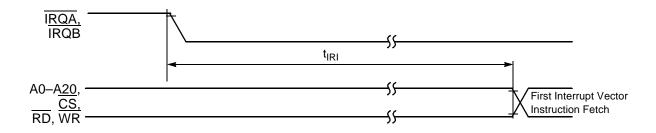
Figure 15. Interrupt from Wait State Timing
