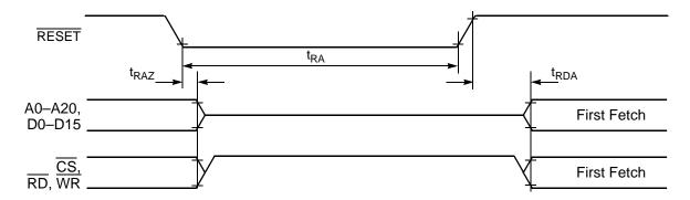
Figure 12. Asynchronous Reset Timing
