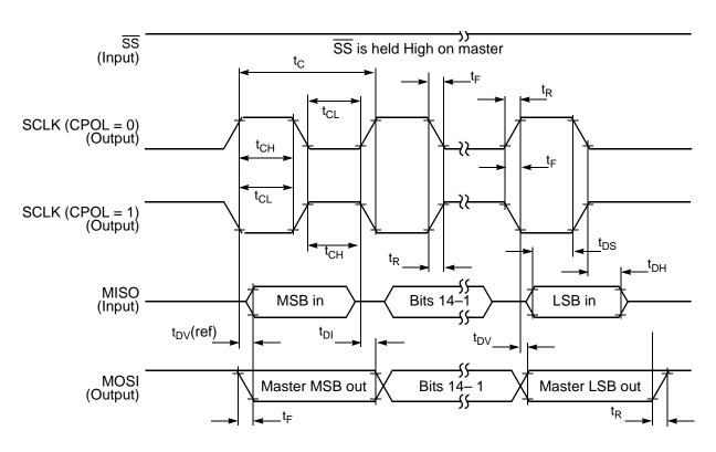
Figure 19. SPI Master Timing (CPHA = 1)
