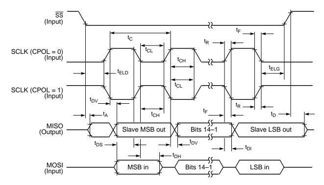
Figure 21. SPI Slave Timing (CPHA = 1)
