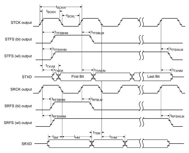
Figure 23. Master Mode Timing Diagram
