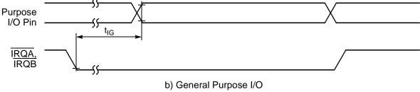
Figure 14. External Level-Sensitive Interrupt Timing
