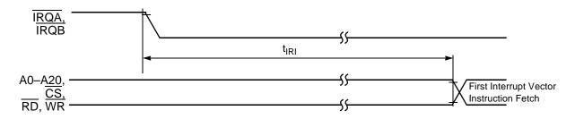
Figure 15. Interrupt from Wait State Timing
