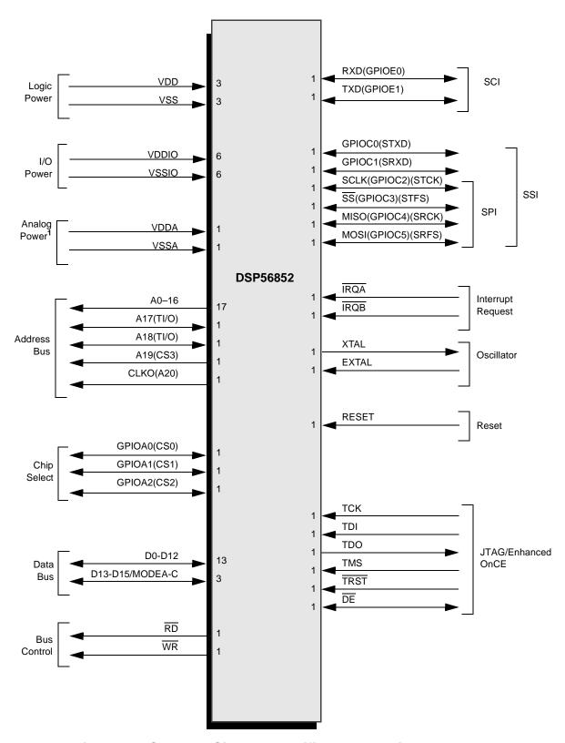
Figure 2. DSP56852 Signals Identified by Functional Group
