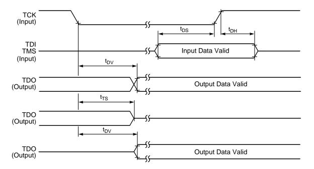
Figure 29. Test Access Port Timing Diagram
