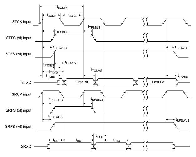
Figure 24. Slave Mode Clock Timing
