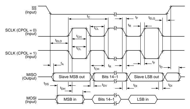
Figure 20. SPI Slave Timing (CPHA = 0)
