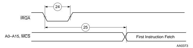
**Figure 2-9** Recovery from Stop Using  $\overline{IRQA}$
