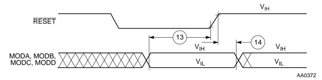
Figure 2-8 Operating Mode Select Timing
