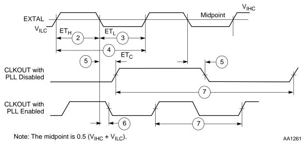
Figure 2-2 External Clock Timing
