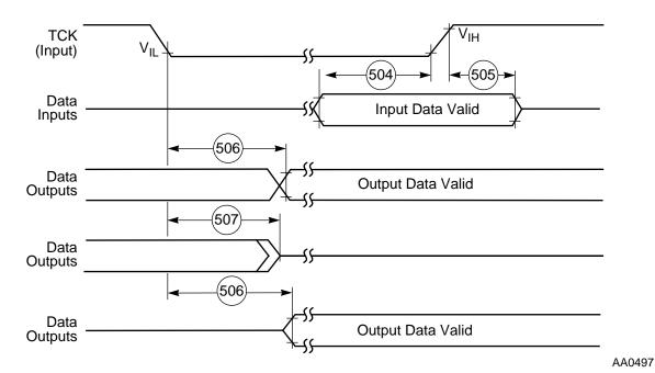
Figure 2-26 Boundary Scan (JTAG) Timing Diagram
