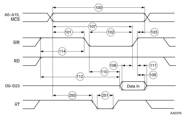
Figure 2-12 SRAM Write Access
