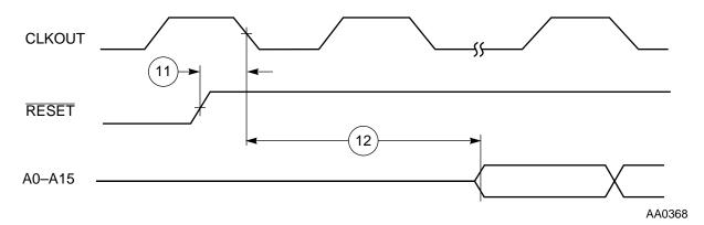
Figure 2-4 Synchronous Reset Timing
