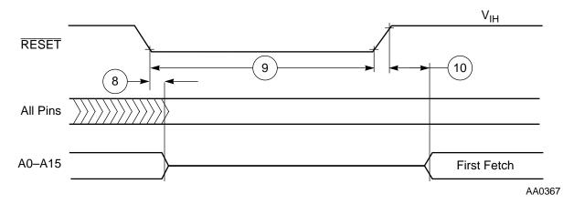
Figure 2-3 Reset Timing
