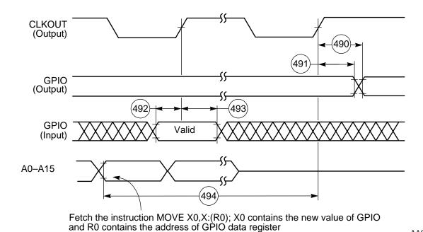
Figure 2-24 GPIO Timing
