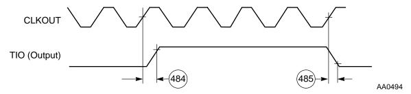
Figure 2-23 External Pulse Generation
