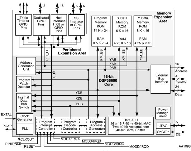
Figure 1 DSP56602 Block Diagram
