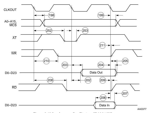
Figure 2-13 Synchronous Bus Timings SRAM 1 WS
