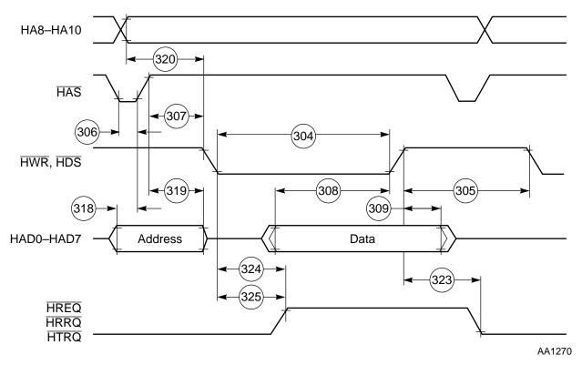
Figure 2-18 Write Timing Diagram—Multiplexed Bus
