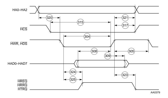
Figure 2-15 Write Timing Diagram—Non-Multiplexed Bus
