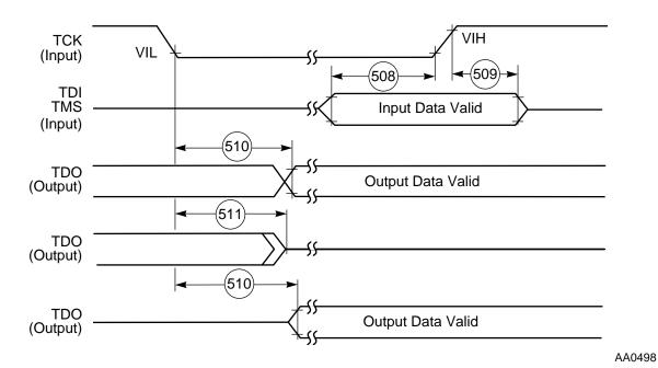
Figure 2-27 Test Access Port Timing Diagram
