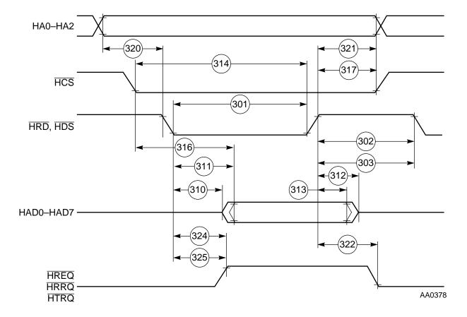
Figure 2-14 Read Timing Diagram—Non-Multiplexed Bus
