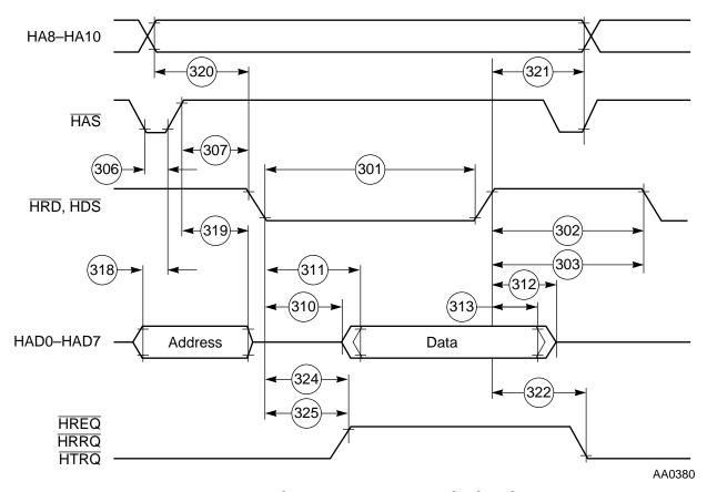
Figure 2-17 Read Timing Diagram—Multiplexed Bus
