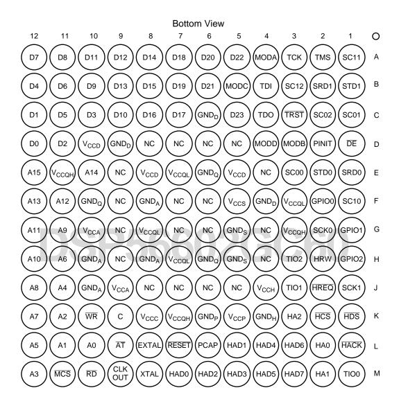
Figure 3-5 Bottom View, DSP56602 PBGA Package
