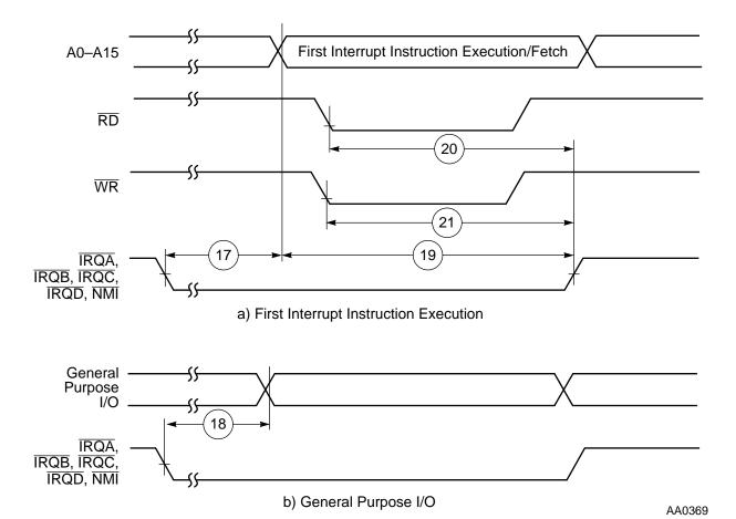
Figure 2-5 External Level-Sensitive Fast Interrupt Timing
