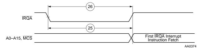
Figure 2-10 Recovery from Stop Using  $\overline{IRQA}$  Interrupt Service
