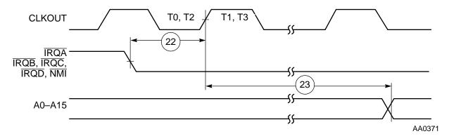
Figure 2-7 Synchronous Interrupt from Wait Timing
