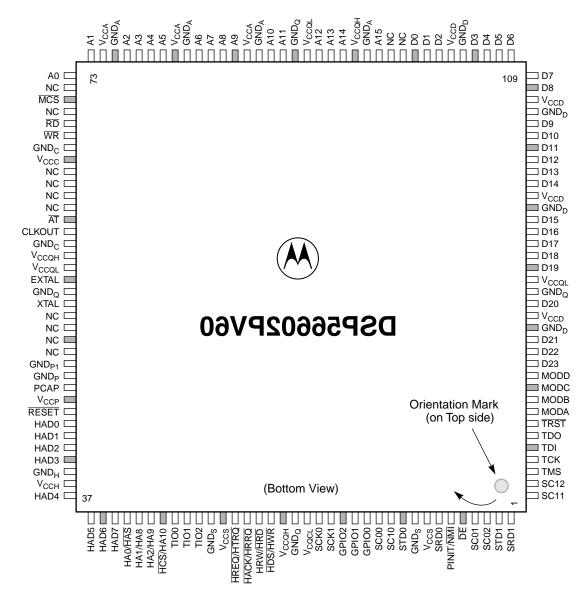
Notes: 1. Pins marked "NC" are no connection pins that are reserved for possible future enhancements. Do not connect these pins to any power, ground, signal traces, or vias.
