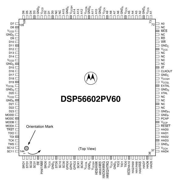
Notes: 1. Pins marked "NC" are no connection pins that are reserved for possible future enhancements. Do not connect these pins to any power, ground, signal traces, or vias.
