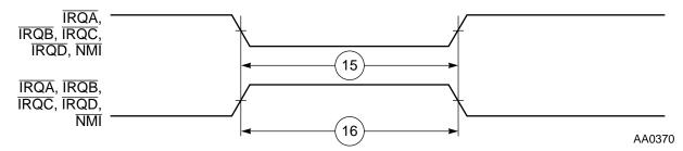
Figure 2-6 External Interrupt Timing (Negative-Edge-Triggered)
