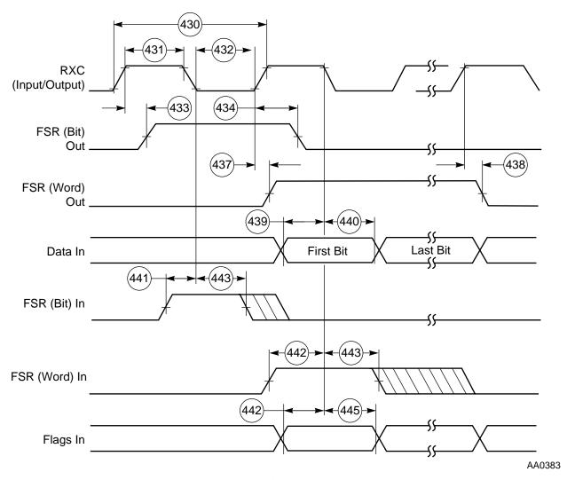
Figure 2-20 SSI Receiver Timing
