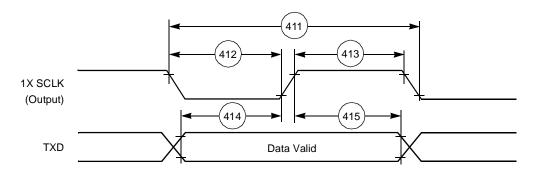
Figure 2-23. SCI Asynchronous Mode Timing
