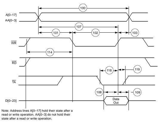
Figure 2-11. SRAM Write Access
