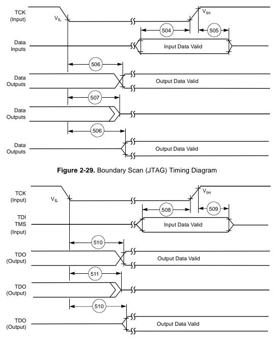
Figure 2-30. Test Access Port Timing Diagram
