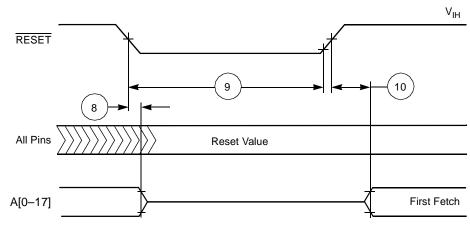
Figure 2-3. Reset Timing
