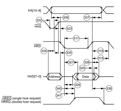
Figure 2-19. Read Timing Diagram, Multiplexed Bus, Double Data Strobe
