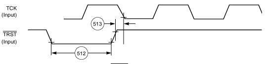
Figure 2-31. TRST Timing Diagram
