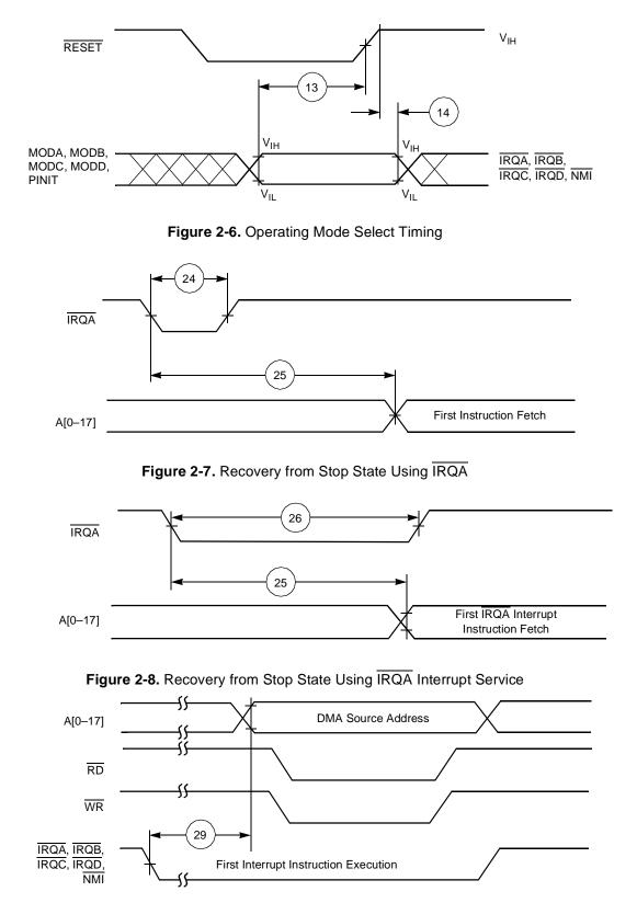
Figure 2-9. External Memory Access (DMA Source) Timing
