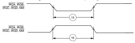
Figure 2-5. External Interrupt Timing (Negative Edge-Triggered)
