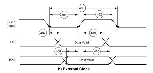
Figure 2-22. SCI Synchronous Mode Timing
