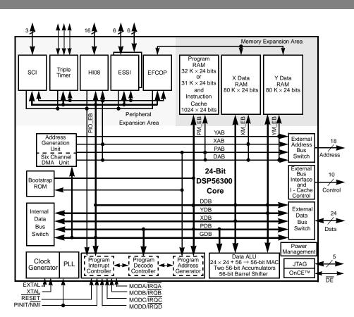
Figure 1. DSP56321 Block Diagram
