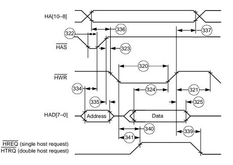
Figure 2-21. Write Timing Diagram, Multiplexed Bus, Double Data Strobe
