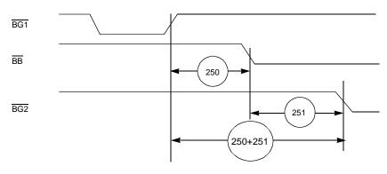
Figure 2-12. Asynchronous Bus Arbitration Timing
