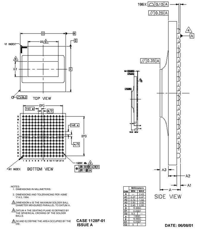
Figure 3-3. DSP56321 Mechanical Information, 196-pin FC-PBGA Package
