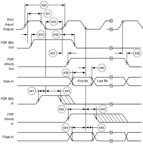
Figure 2-25. ESSI Receiver Timing
