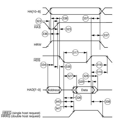
Figure 2-18. Read Timing Diagram, Multiplexed Bus, Single Data Strobe
