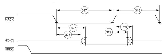
Figure 2-20. Host Interrupt Vector Register (IVR) Read Timing Diagram
