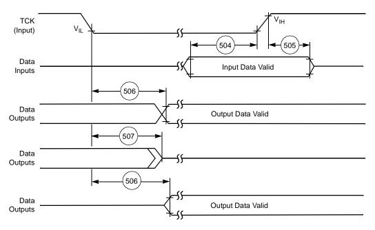
Figure 2-36. Boundary Scan (JTAG) Timing Diagram
