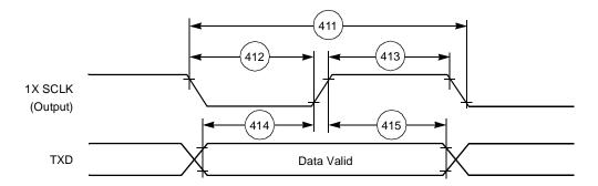
Figure 2-30. SCI Asynchronous Mode Timing
