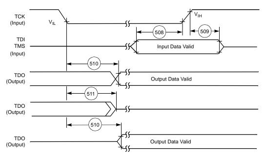
Figure 2-37. Test Access Port Timing Diagram
