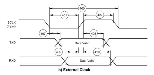
Figure 2-29. SCI Synchronous Mode Timing
