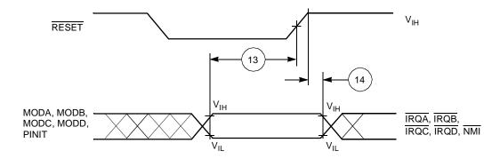
Figure 2-6. Operating Mode Select Timing
