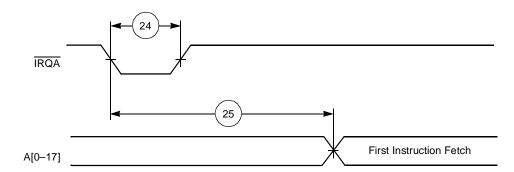
Figure 2-7. Recovery from Stop State Using IRQA
