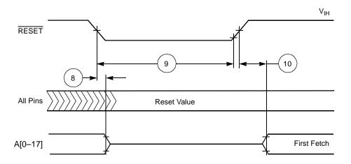
Figure 2-3. Reset Timing
