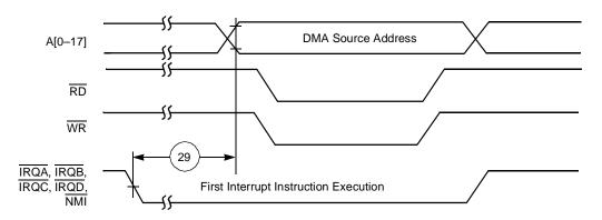
Figure 2-9. External Memory Access (DMA Source) Timing
