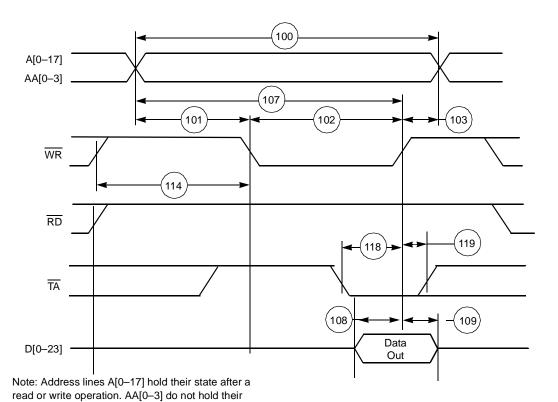
Figure 2-11. SRAM Write Access
