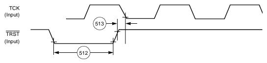
Figure 2-38. TRST Timing Diagram
