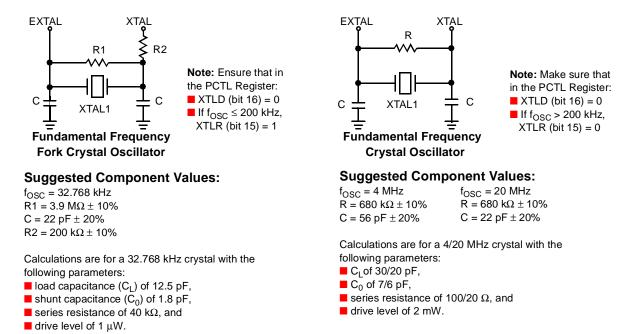
Figure 2-1. Crystal Oscillator Circuits
