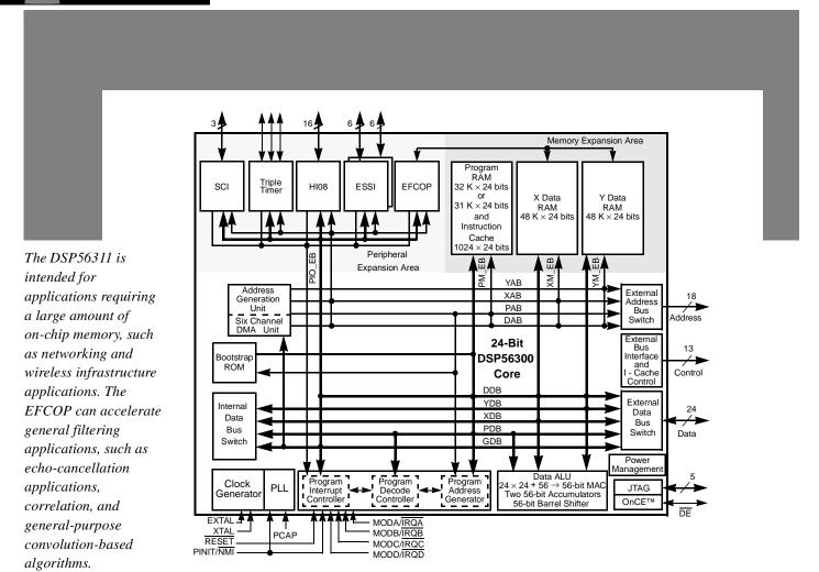
Figure 1. DSP56311 Block Diagram
