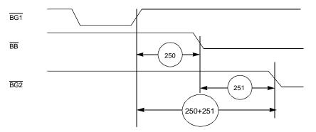
Figure 2-19. Asynchronous Bus Arbitration Timing
