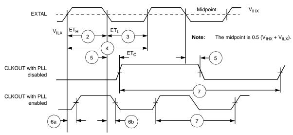
Figure 2-2. External Clock Timing
