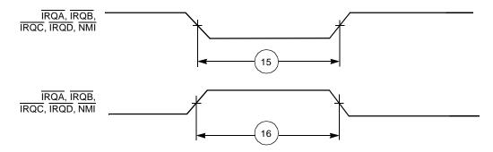
Figure 2-5. External Interrupt Timing (Negative Edge-Triggered)
