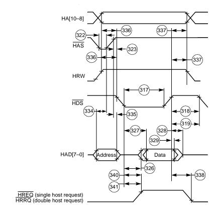
Figure 2-25. Read Timing Diagram, Multiplexed Bus, Single Data Strobe
