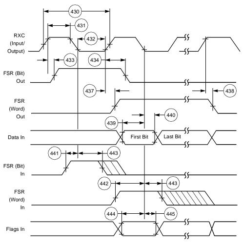
Figure 2-32. ESSI Receiver Timing
