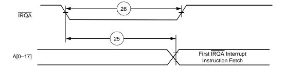
Figure 2-8. Recovery from Stop State Using IRQA Interrupt Service
