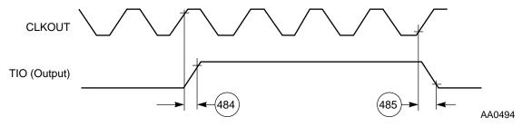
Figure 2-39 External Pulse Generation
