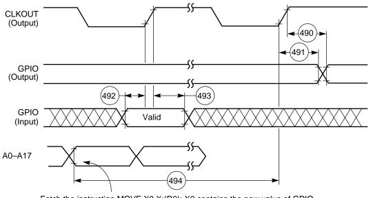
Fetch the instruction MOVE X0,X:(R0); X0 contains the new value of GPIO and R0 contains the address of GPIO data register.
