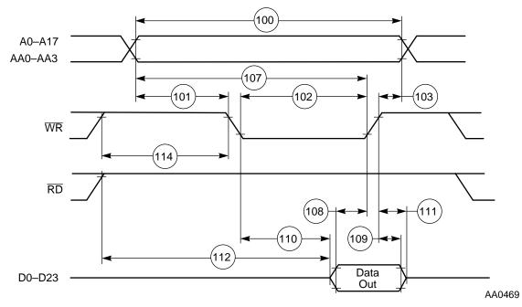
Figure 2-13 SRAM Write Access
