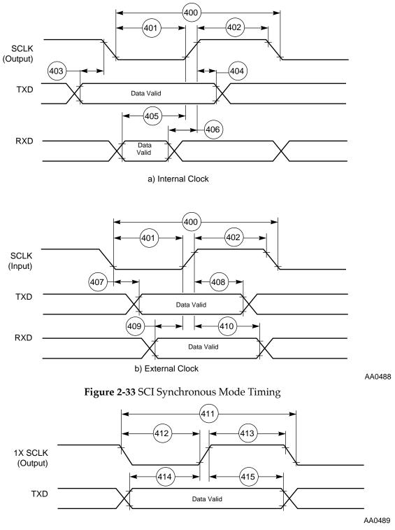
Figure 2-34 SCI Asynchronous Mode Timing
