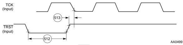
Figure 2-44 TRST Timing Diagram
