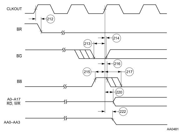
Figure 2-23 Bus Acquisition Timings
