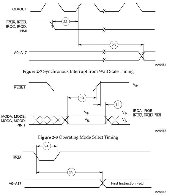
Figure 2-9 Recovery from Stop State Using IRQA
