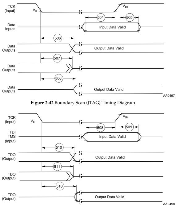
Figure 2-43 Test Access Port Timing Diagram
