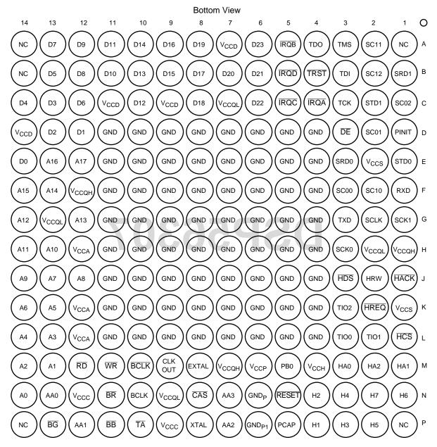
Figure 3-2 DSP56307 Plastic Ball Grid Array (PBGA), Bottom View
