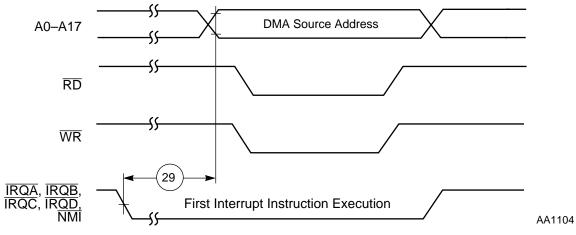
Figure 2-11 External Memory Access (DMA Source) Timing
