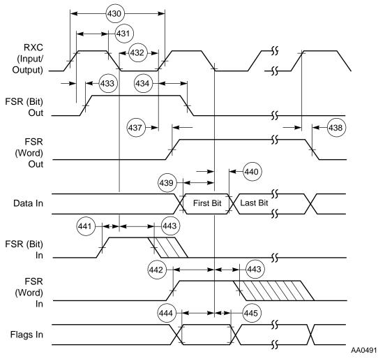
Figure 2-36 ESSI Receiver Timing
