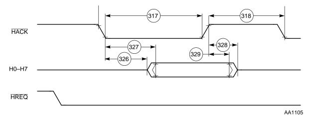
Figure 2-28 Host Interrupt Vector Register (IVR) Read Timing Diagram
