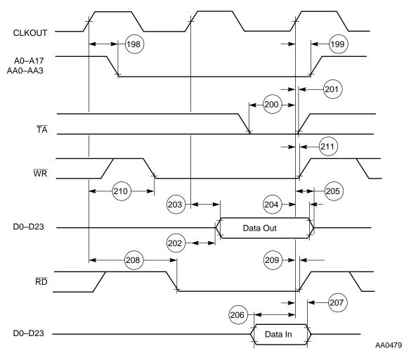
Figure 2-21 Synchronous Bus Timings 1 WS (BCR Controlled)
