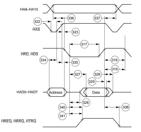
Figure 2-31 Read Timing Diagram, Multiplexed Bus
