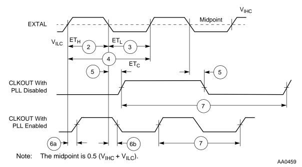
Figure 2-2 External Clock Timing
