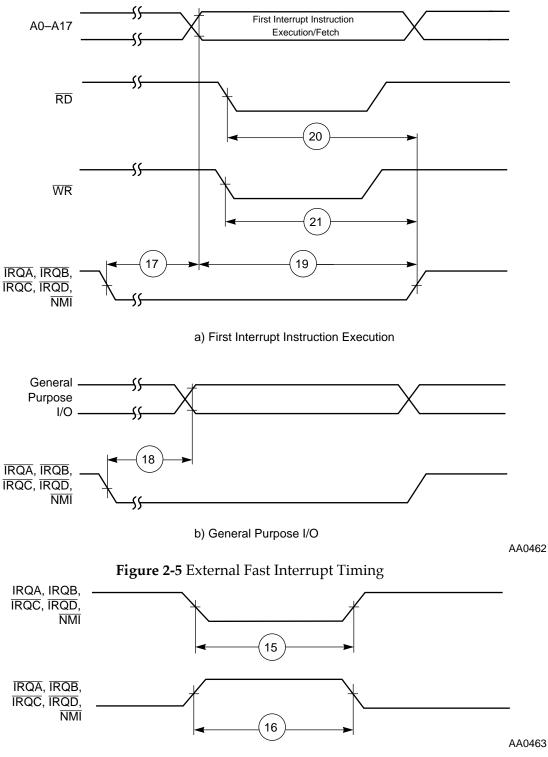
Figure 2-6 External Interrupt Timing (Negative Edge-Triggered)
