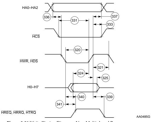
Figure 2-30 Write Timing Diagram, Non-Multiplexed Bus
