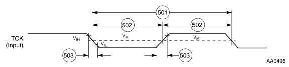
Figure 2-41 Test Clock Input Timing Diagram
