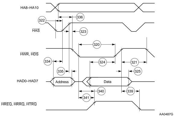
Figure 2-32 Write Timing Diagram, Multiplexed Bus
