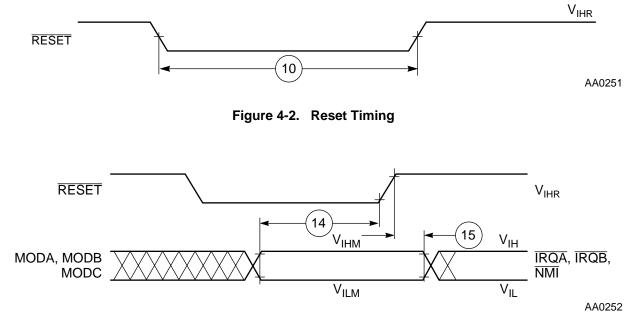
Figure 4-3. Operating Mode Select Timing
