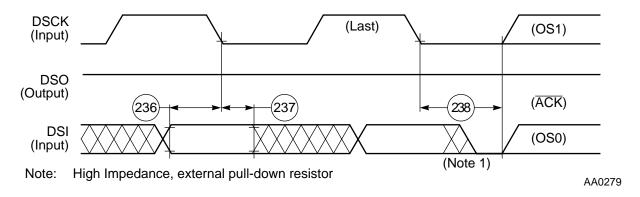
Figure 4-24. DSP56012 OnCE Data I/O to Status Timing
