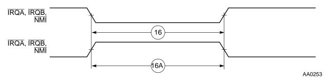
Figure 4-4. External Interrupt Timing (Negative-Edge Triggered)
