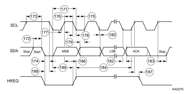
Figure 4-19. I<sup>2</sup>C Timing
