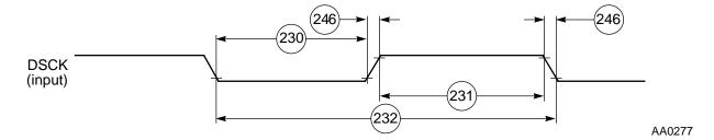
Figure 4-22. DSP56012 OnCE Serial Clock Timing
