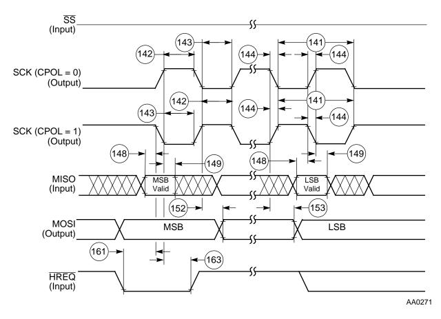
Figure 4-15. SPI Master Timing (CPHA = 0)
