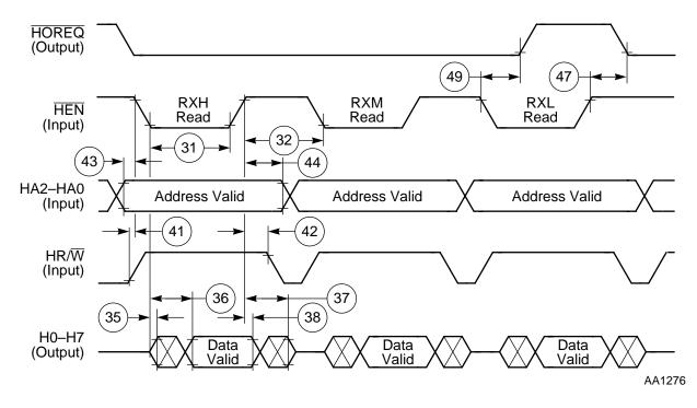
Figure 4-9. Host Read Cycle (Non-DMA Mode)
