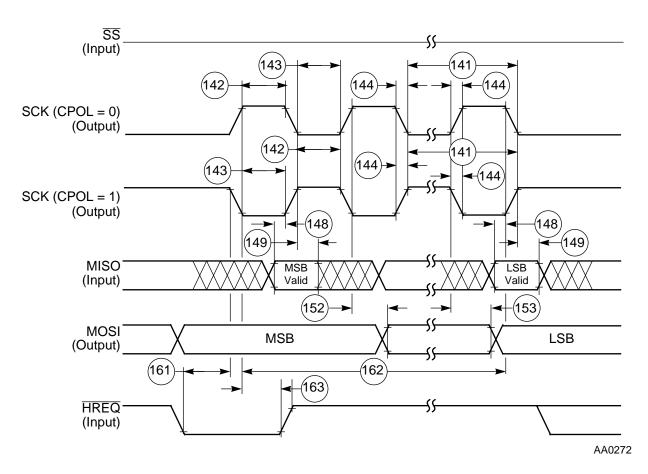
Figure 4-16. SPI Master Timing (CPHA = 1)
