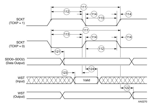
Figure 4-14. SAI Transmitter Timing
