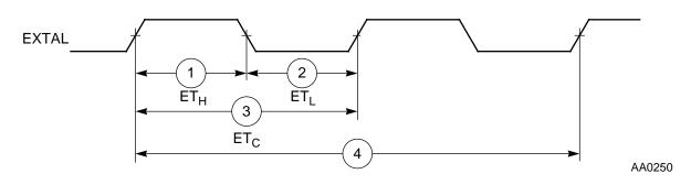
Figure 4-1. External Clock Timing
