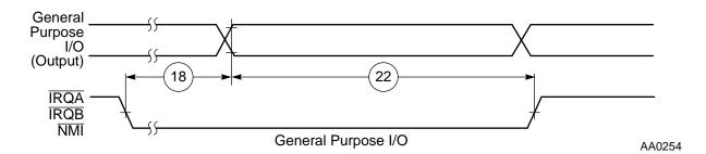
Figure 4-5. External Level-Sensitive Fast Interrupt Timing
