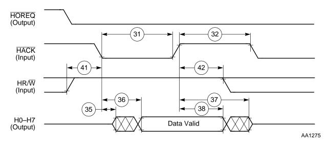
Figure 4-8. Host Interrupt Vector Register (IVR) Read
