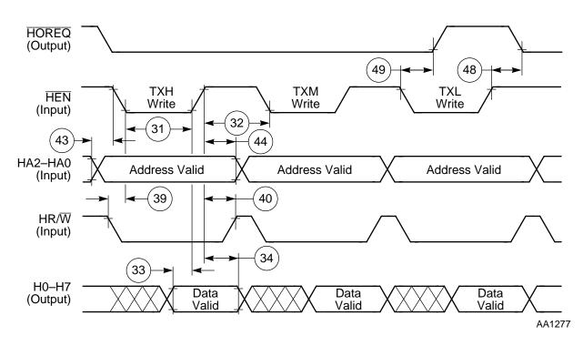
Figure 4-10. Host Write Cycle (Non-DMA Mode)
