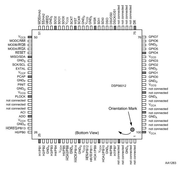
Figure 5-2. DSP56012 Thin Quad Flat Pack (TQFP), Bottom View
