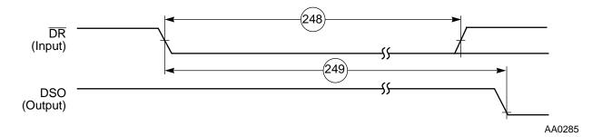
Figure 4-30. Asynchronous Recovery from Wait State
