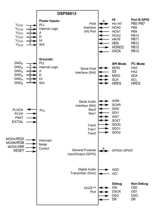
Figure 3-1. Signals Identified by Functional Group
