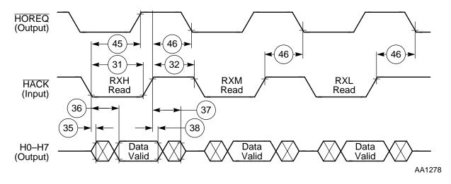
Figure 4-11. Host DMA Read Cycle
