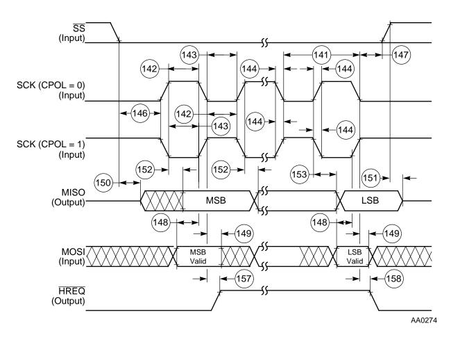
Figure 4-18. SPI Slave Timing (CPHA = 1)
