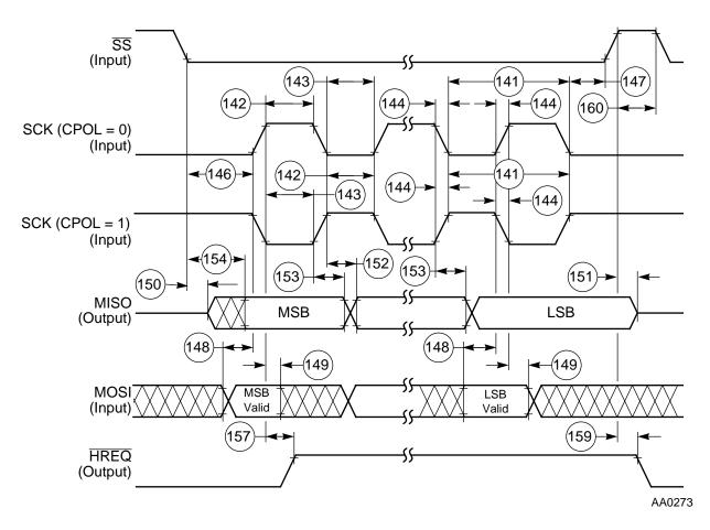
Figure 4-17. SPI Slave Timing (CPHA = 0)
