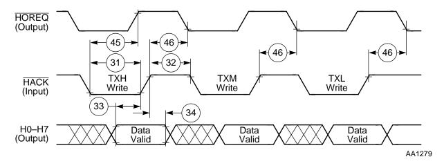
Figure 4-12. Host DMA Write Cycle
