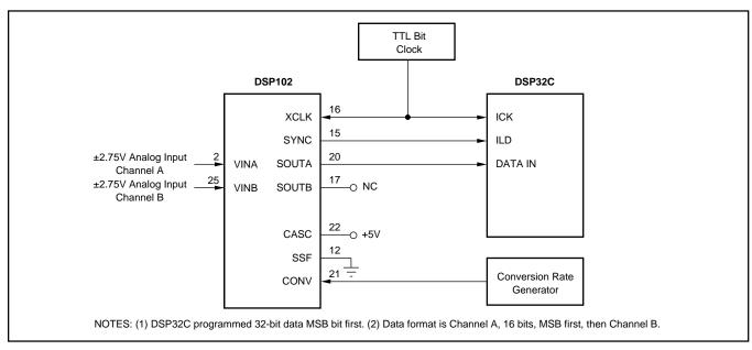
FIGURE 21. Using DSP102 with DSP32C in Cascade Mode.
