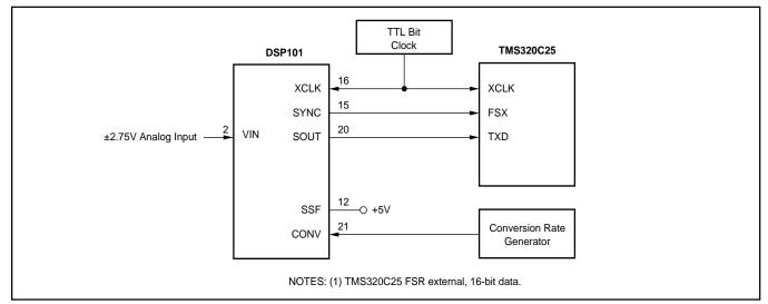
FIGURE 16. Using DSP101 with TMS320C25.
