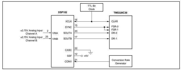
FIGURE 12. Using DSP102 with TMS320C30.
