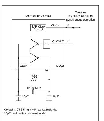
FIGURE 5. DSP101 or DSP102 Conversion Clock Circuit.
