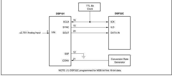
FIGURE 19. Using DSP101 with DSP32C.
