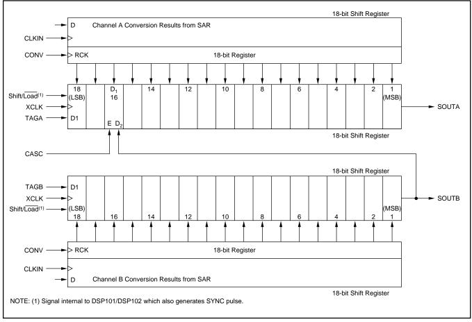
FIGURE 4. Output Structure of DSP102.
