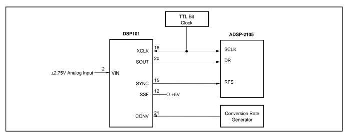
FIGURE 23. Using DSP101 with ADSP-2105.
