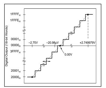
FIGURE 3. Analog Input to Digital Output Diagram.
