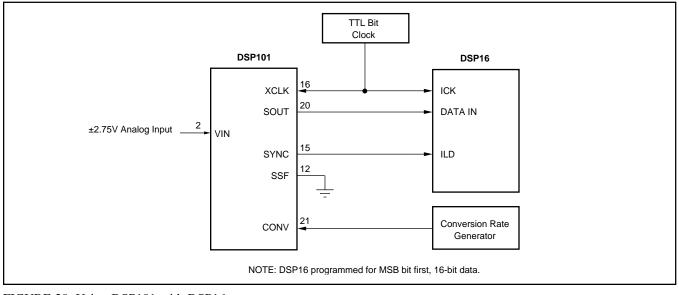
FIGURE 20. Using DSP101 with DSP16.
