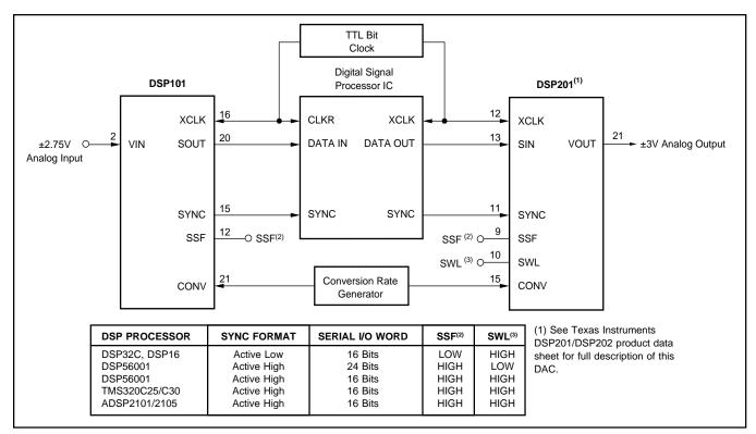
FIGURE 11. Analog Input and Analog Output System.
