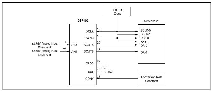
FIGURE 22. Using DSP102 with ADSP-2101.
