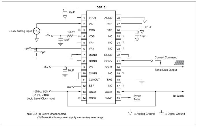
FIGURE 2. DSP101 Basic Operation.
