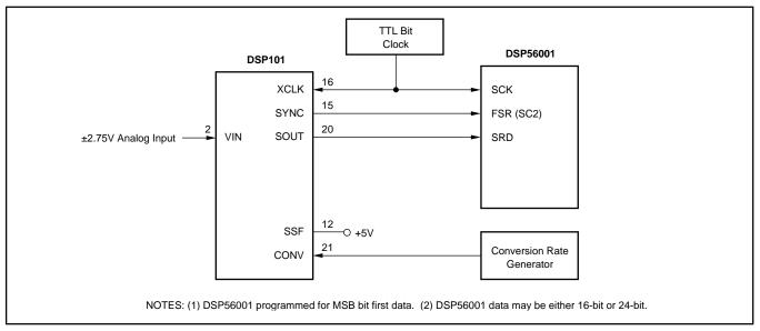
FIGURE 18. Using DSP101 with DSP56001.
