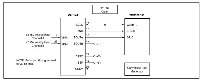
FIGURE 13. Using DSP102 with TMS320C30 in Cascade Mode.
