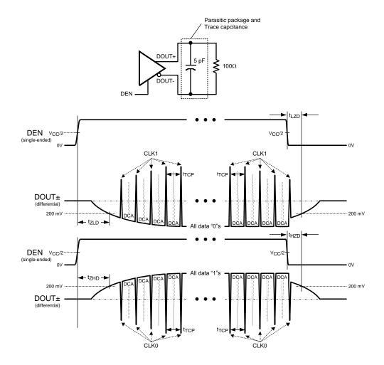
Figure 6. Serializer TRI-STATE Test Circuit and Delay
