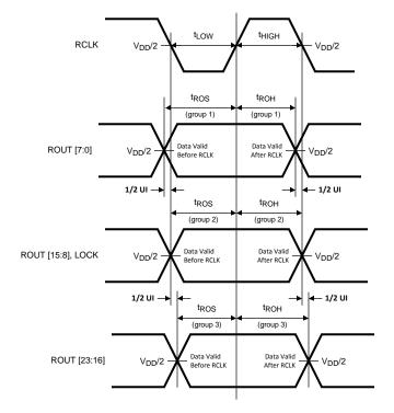
Figure 15. Deserializer Setup and Hold Times
