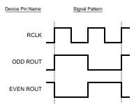
Figure 2. Deserializer Output Checker-board Pattern
