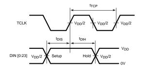
Figure 5. Serializer Setup/Hold Times
