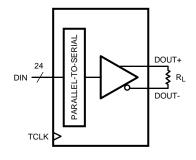
$\label{eq:VOD} VOD = (D_{OUT+}) - (D_{OUT-})$  Differential output signal is shown as (D\_{OUT+}) - (D\_{OUT-}), device in Data Transfer mode.
