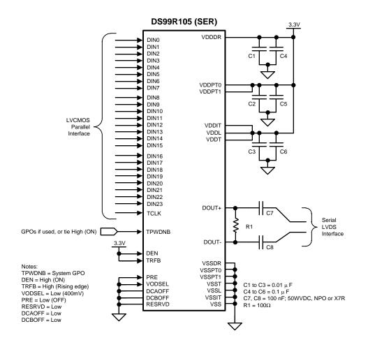
Figure 20. DS99R105 Typical Application Connection
