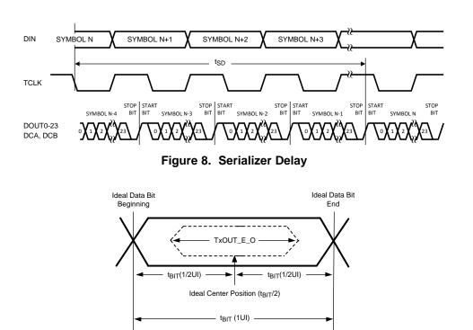
Figure 9. Transmitter Output Eye Opening (TxOUT\_E\_O)
