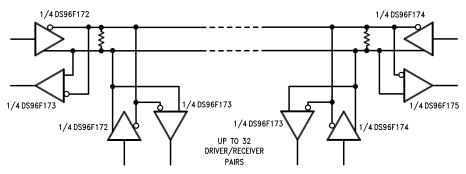
The line length should be terminated at both ends in its characteristic impedance. Stub lengths off the main line should be kept as short as possible.
