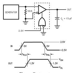
Figure 7.  $t_{PLH}$ ,  $t_{PHL}$
