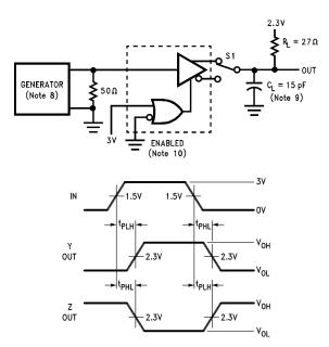
**Note 8:**The input pulse is supplied by a generator having the following characteristics: f = 1.0 MHz, duty cycle = 50%,  $t_f \le 5.0$  ns,  $t_f \le 5.0$  ns,  $Z_O = 50\Omega$ .
