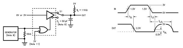
**Note 8:**The input pulse is supplied by a generator having the following characteristics: f = 1.0 MHz, duty cycle = 50%,  $t_f \le 5.0$  ns,  $t_f \le 5.0$  ns,  $Z_O = 50\Omega$ .
