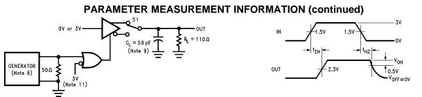
**Note 8:**The input pulse is supplied by a generator having the following characteristics: f = 1.0 MHz, duty cycle = 50%,  $t_f \le 5.0$  ns,  $t_f \le 5.0$  ns,  $Z_O = 50\Omega$ .
