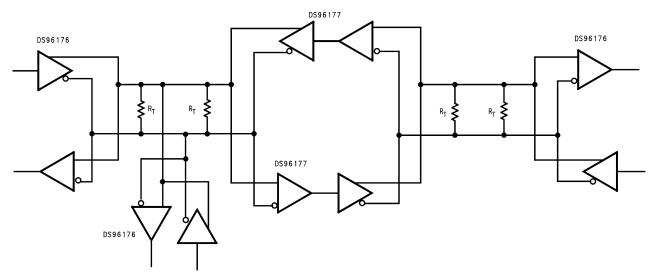
The line length should be terminated at both ends in its characteristic impedance. Stub lengths off the main line should be kept as short as possible. Repeater control logic not shown
