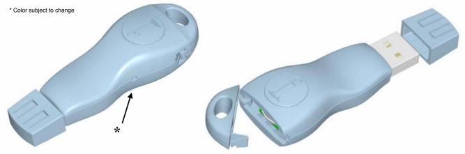
\*Note: To eject an <u>i</u>Button, insert a straightened paper clip into the side access hole of the DS9490B. Push the paper clip in the direction of the <u>i</u>Button. A different <u>i</u>Button can then be inserted. The data contact faces down and away from the embossed 'i'. Before inserting the paper clip disconnect the DS9490B from the USB bus.
