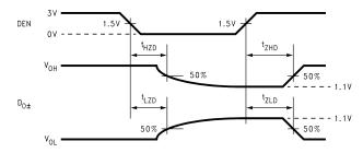
Figure 5. Serializer Input Clock Transition Time TRI-STATE Test Circuit and Timing
