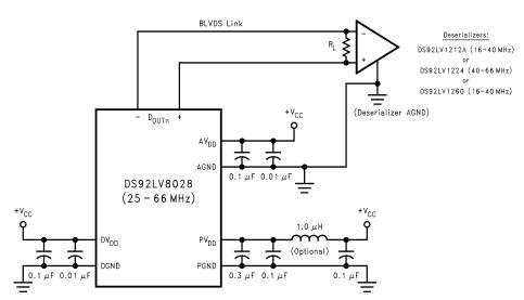
Figure 12. Typical Application Circuit
