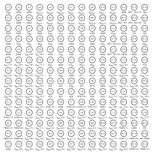
Figure 13. Top View of DS92LV8028 (196-pin NFBGA)
