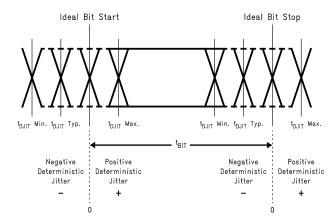
Figure 9. Deterministic Jitter and Ideal Bit Position
