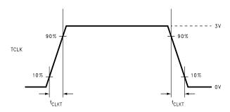
Figure 3. Serializer Input Clock Transition Time
