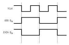
Figure 1. 'Worst Case Icc Test Pattern
