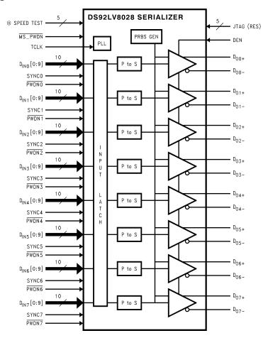
Figure 11. DS92LV8028 Functional Block Diagram
