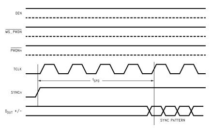
Figure 8. SYNC Timing Delays
