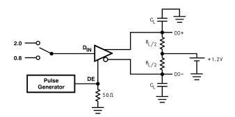
Figure 4. Driver TRI-STATE Delay Test Circuit
