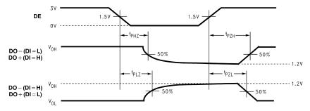
Figure 5. Driver TRI-STATE Delay Waveforms
