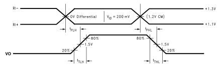
Figure 7. Receiver Propagation Delay and Transition Time Waveforms
