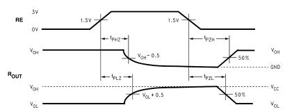
Figure 9. Receiver TRI-STATE Delay Waveforms TRI-STATE Delay Waveforms
