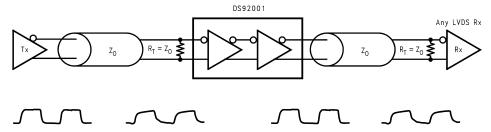
Figure 11. Cable Repeater Application
