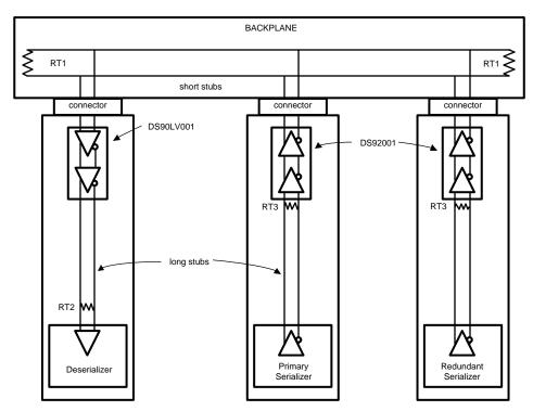
Figure 10. Backplane Stub-Hider Application
