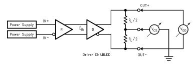
Figure 3. Differential Driver DC Test Circuit
