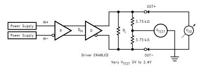
Figure 4. Differential Driver Full Load DC Test Circuit
