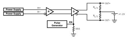
Figure 8. TRI-STATE Delay Test Circuit
