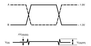
Figure 2. Differential Driver Waveforms
