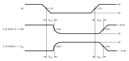
Figure 9. Driver TRI-STATE Delay Waveforms
