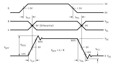
Figure 7. Driver Propagation Delays and Transition Time Waveforms
