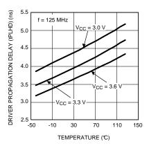
Figure 13. Driver Propagation Delay (tPLHD) as a Function of Temperature
