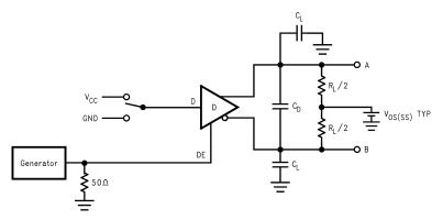
Figure 8. Driver TRI-STATE Delay Test Circuit
