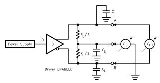
Figure 1. Differential Driver Test Circuit
