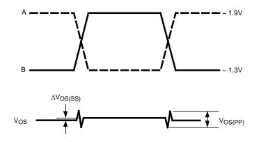
Figure 2. Differential Driver Waveforms
