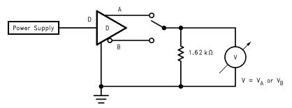
Figure 4. Differential Driver DC Open Test Circuit
