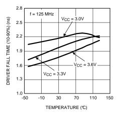
Figure 11. Driver Fall Time as a Function of Temperature
