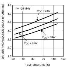
Figure 13. Driver Propagation Delay (tPLHD) as a Function of Temperature
