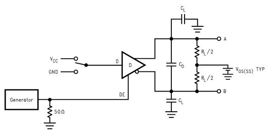
Figure 8. Driver TRI-STATE Delay Test Circuit
