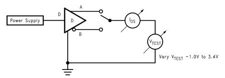
Figure 5. Differential Driver Short-Circuit Test Circuit
