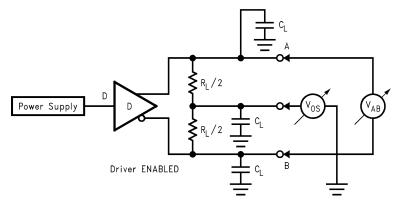
Figure 1. Differential Driver Test Circuit
