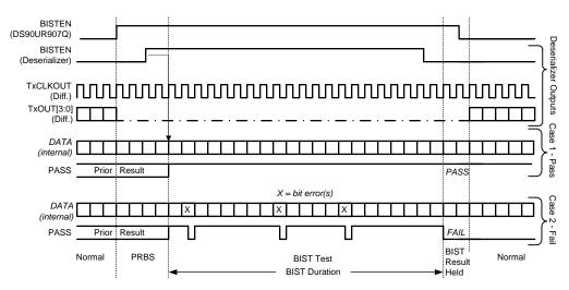
Figure 21. BIST Waveforms
