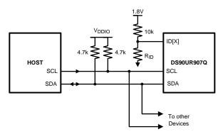
Figure 22. Serial Control Bus Connection
