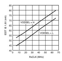
Figure 14. Typical IDDT (1.8V Supply) Current as a function of RxCLK
