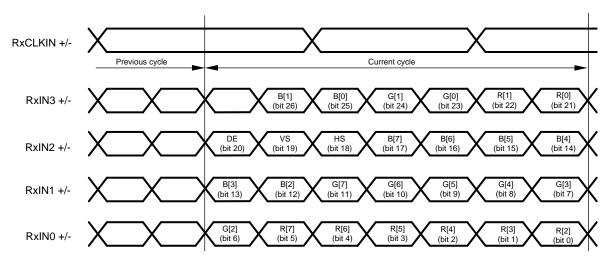
Figure 17. 8-bit FPD-LInk Mapping: LSB's on RxIN3
