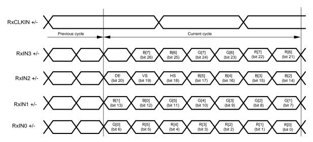
Figure 18. 8-bit FPD-LInk Mapping: MSB's on RxIN3
