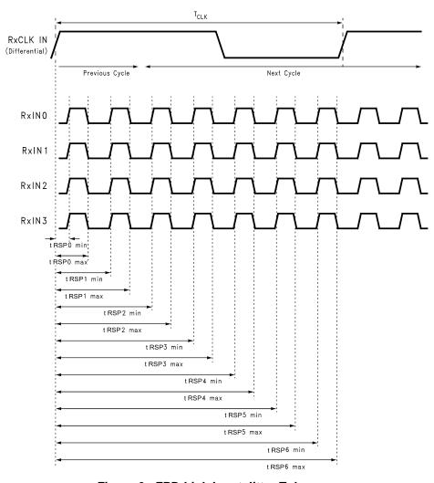
Figure 6. FPD-Link Input Jitter Tolerance
