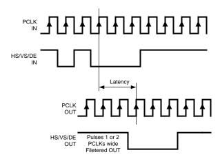
Figure 16. Video Control Signal Filter Wavefrom
