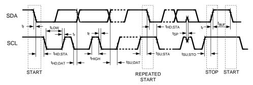
Figure 13. Serial Control Bus Timing Diagram
