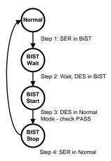
Figure 20. BIST Mode Flow Diagram
