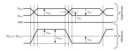
Figure 4. Output Waveforms
