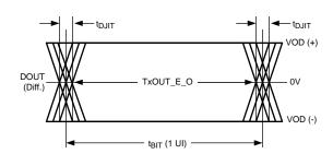
Figure 10. Output Jitter
