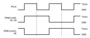
Figure 3. Checkboard Data Pattern
