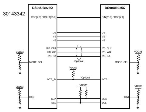
Figure 15. Repeater Connection Diagram
