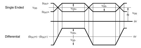
Figure 2. Serializer VOD DC Output
