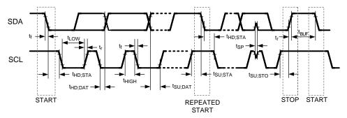
Figure 9. Serial Control Bus Timing Diagram
