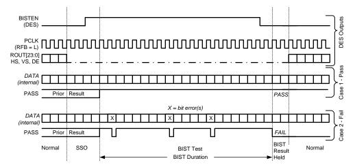
Figure 17. BIST Waveforms
