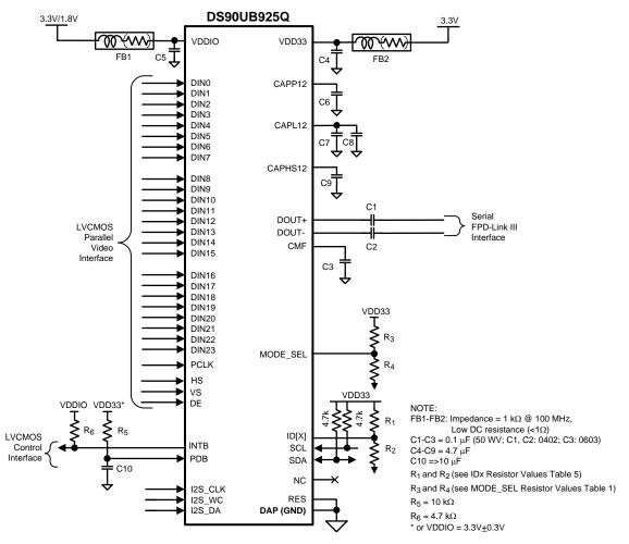
Figure 22. Typical Connection Diagram
