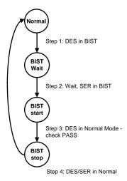
Figure 16. BIST Mode Flow Diagram
