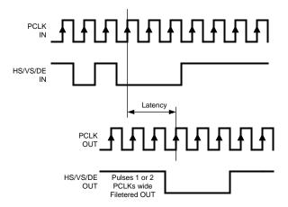
Figure 11. Video Control Signal Filter Waveform
