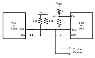
Figure 18. Serial Control Bus Connection
