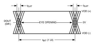
Figure 8. Serializer CML Output Jitter
