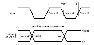
Figure 6. Serializer Setup and Hold Times
