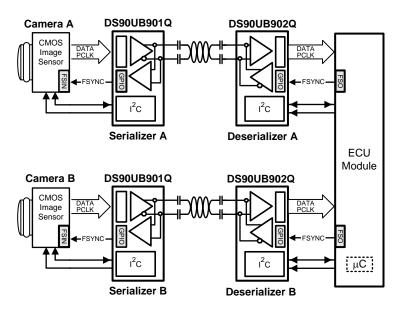
Figure 32. Synchronizing Multiple Cameras
