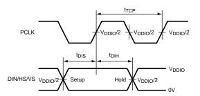
Figure 12. Serializer Setup/Hold Times
