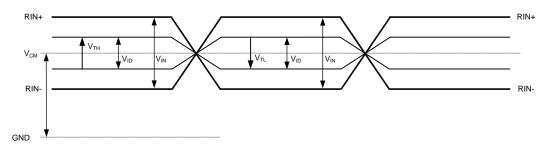
Figure 10. Differential VTH/VTL Definition Diagram
