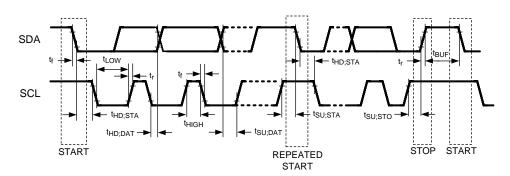
Figure 4. Bidirectional Control Bus Timing
