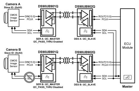
Figure 31. I<sup>2</sup>C Pass Through
