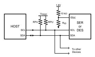
Figure 28. Bidirectional Control Bus Connection
