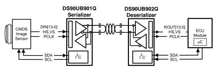
Figure 29. Typical Camera System Diagram
