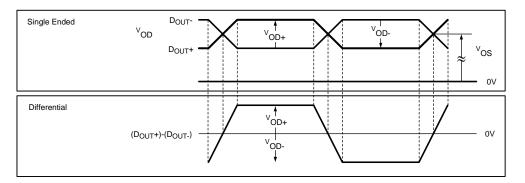
Figure 9. Serializer VOD DC Diagram
