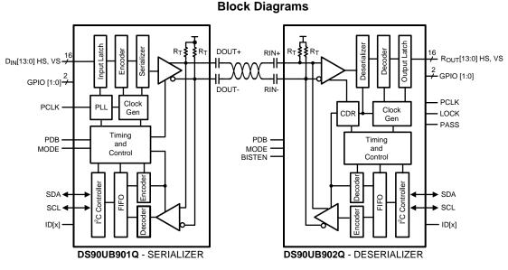
Figure 2. Block Diagram
