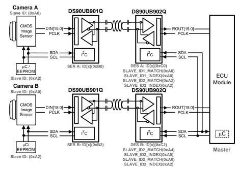
Figure 30. Multiple Device Addressing
