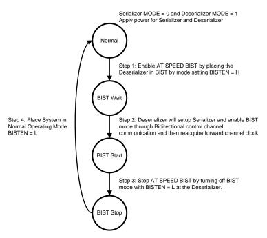
Figure 34. AT-SPEED BIST System Flow Diagram
