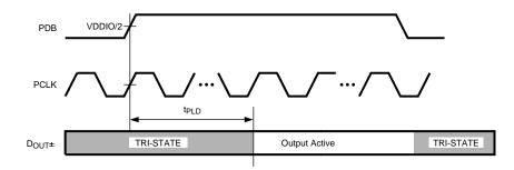
Figure 13. Serializer Data Lock Time
