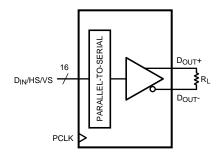
Figure 8. Serializer VOD DC Diagram
