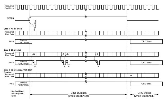
Figure 35. BIST Timing Diagram
