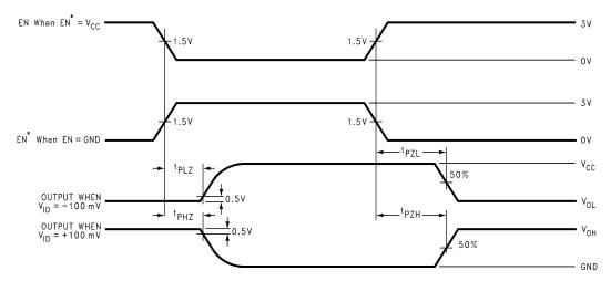
Figure 4. Receiver TRI-STATE Delay Waveforms
