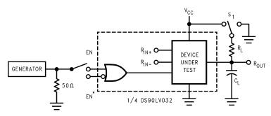
C<sub>L</sub> includes load and test jig capacitance.
