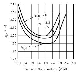
Figure 9. Variation in Low to High Propagation Delay versus  $V_{\text{CM}}$
