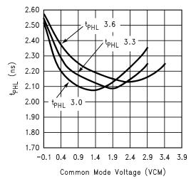
Figure 8. Variation in High to Low Propagation Delay versus  $V_{\text{CM}}$
