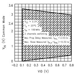
Figure 6. Typical Common-Mode Range variation with respect to amplitude of differential input
