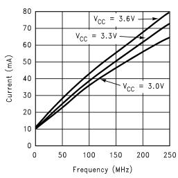
Figure 5. I<sub>CC</sub> vs Frequency, four channels switching
