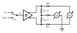
Figure 2. Differential Driver DC Test Circuit
