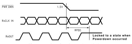
Figure 19. Receiver Powerdown Delay
