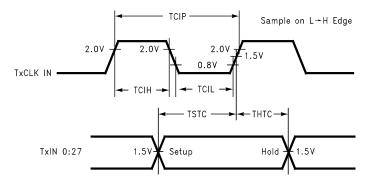
Figure 9. DS90CR583 (Transmitter) Setup/Hold and High/Low Times
