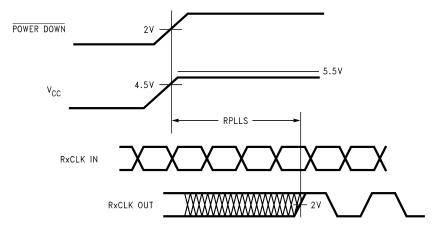
Figure 14. DS90CR584 (Receiver) Phase Lock Loop Set Time
