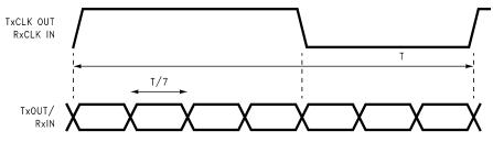
Figure 17. Seven Bits of LVDS in One Clock Cycle
