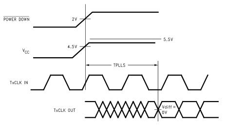
Figure 13. DS90CR583 (Transmitter) Phase Lock Loop Set Time
