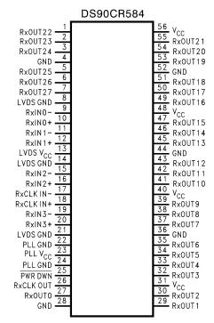
Figure 22. 56 Pin TSSOP See Package Number DGG
