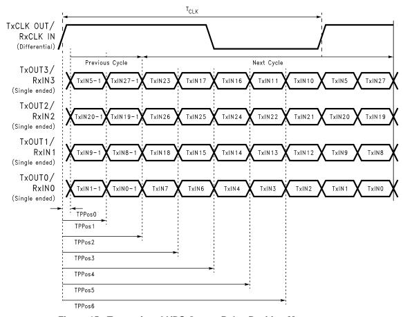
Figure 15. Transmitter LVDS Output Pulse Position Measurement
