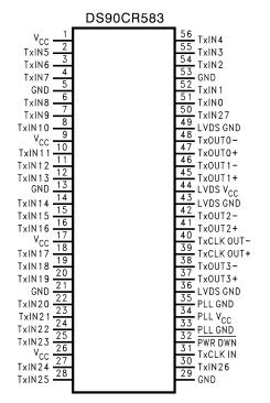
Figure 21. 56 Pin TSSOP See Package Number DGG
