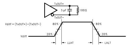
Figure 8. DS90CR561 (Transmitter) LVDS Output Load and Transition Timing
