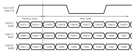
Figure 19. 21 Parallel TTL Data Inputs Mapped to LVDS Outputs (DS90CR561)
