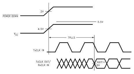
Figure 16. DS90CR561 (Transmitter) Phase Lock Loop Set Time
