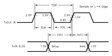
Figure 12. DS90CR561 Setup/Hold and High/Low Times
