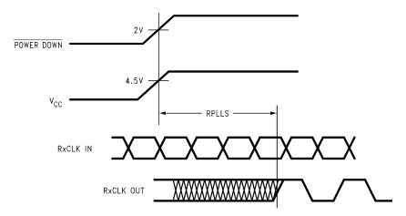
Figure 17. DS90CR562 (Receiver) Phase Lock Loop Set Time
