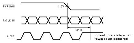
Figure 21. Receiver Powerdown Delay
