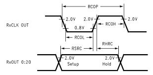
Figure 13. DS90CR562 Setup/Hold and High/Low Times
