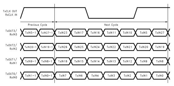
Figure 17. 28 Parallel TTL Data Inputs Mapped to LVDS Outputs
