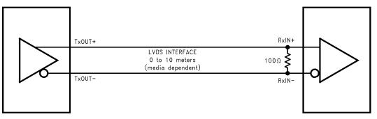
Figure 23. LVDS Serialized Link Termination
