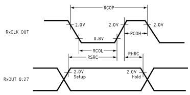
Figure 11. DS90CR286 (Receiver) Setup/Hold and High/Low Times
