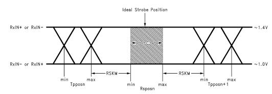
C—Setup and Hold Time (Internal data sampling window) defined by Rspos (receiver input strobe position) min and max
