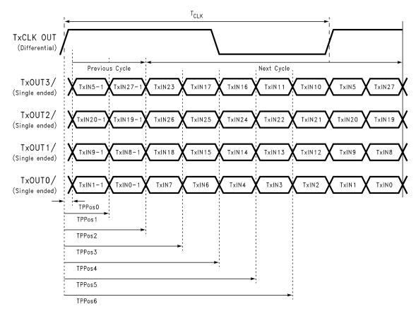
Figure 20. Transmitter LVDS Output Pulse Position Measurement
