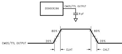
Figure 7. DS90CR286 (Receiver) CMOS/TTL Output Load and Transition Times
