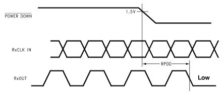
Figure 19. Receiver Powerdown Delay
