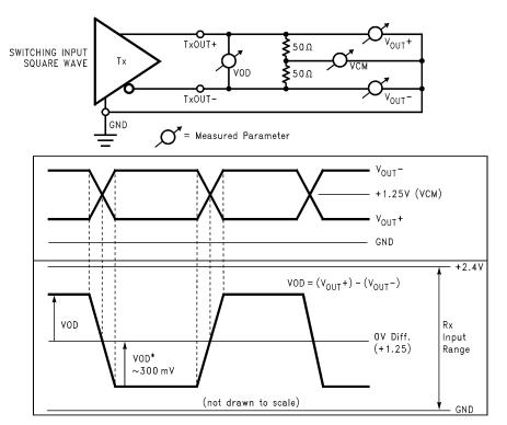
Figure 25. Single-Ended and Differential Waveforms
