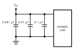
Figure 24. CHANNEL LINK Decoupling Configuration
