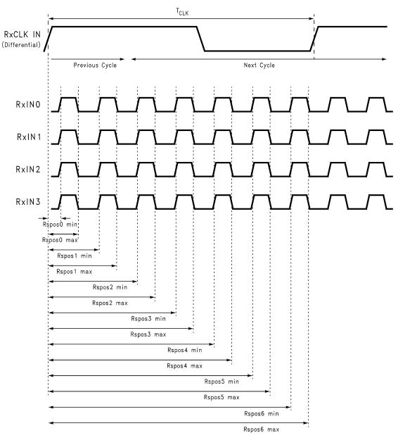
Figure 21. Receiver LVDS Input Strobe Position
