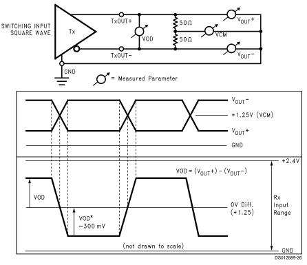
FIGURE 20. Single-Ended and Differential Waveforms
