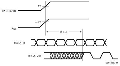
FIGURE 11. DS90CR284 (Receiver) Phase Lock Loop Set Time
