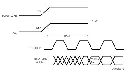
FIGURE 10. DS90CR283 (Transmitter) Phase Lock Loop Set Time
