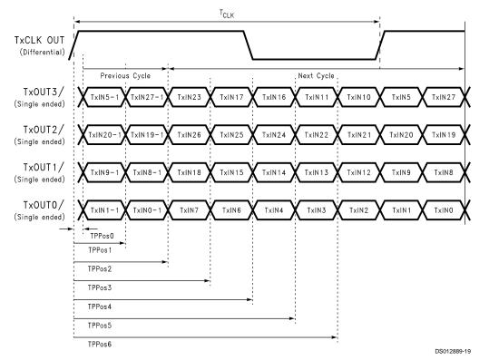
FIGURE 16. Transmitter LVDS Output Pulse Position Measurement
