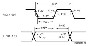
FIGURE 7. DS90CR284 (Receiver) Setup/Hold and High/Low Times
