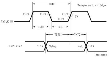
FIGURE 6. DS90CR283 (Transmitter) Setup/Hold and High/Low Times
