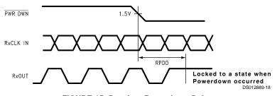
FIGURE 15. Receiver Powerdown Delay
