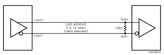
FIGURE 18. LVDS Serialized Link Termination
