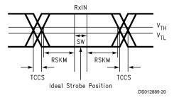
$\ensuremath{\mathsf{SW}} - \ensuremath{\mathsf{Setup}}$  and Hold Time (Internal data sampling window)
