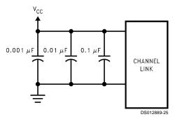
FIGURE 19. CHANNEL LINK Decoupling Configuration
