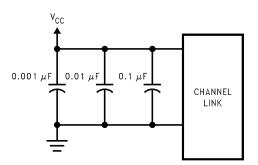
Figure 23. CHANNEL LINK Decoupling Configuration
