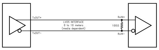
Figure 22. LVDS Serialized Link Termination
