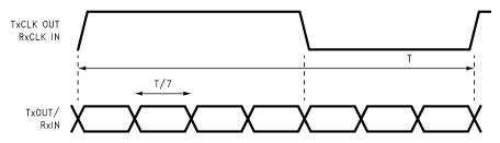
Figure 16. Seven Bits of LVDS in Once Clock Cycle
