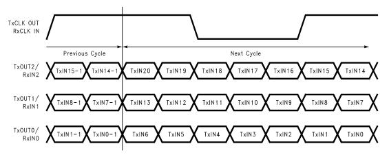
Figure 17. 21 Parallel TTL Data Inputs Mapped to LVDS Outputs
