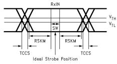
SW—Setup and Hold Time (Internal Data Sampling Window) TCCS—Transmitter Output Skew RSKM ≥ Cable Skew (Type, Length) + Source Clock Jitter (Cycle to Cycle) Cable Skew—Typically 10 ps–40 ps per foot
