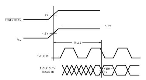
Figure 14. DS90CR213 (Transmitter) Phase Lock Loop Set Time
