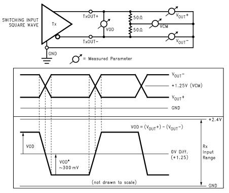
Figure 24. Single-Ended and Differential Waveforms
