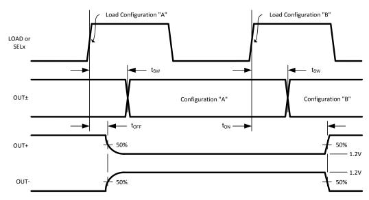
Figure 7. Configuration and Output Enable/Disable Timing
