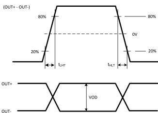
Figure 5. LVDS Output Transition Time
