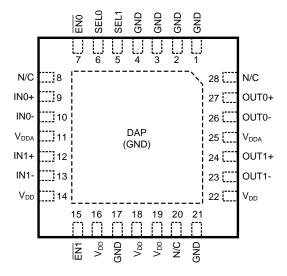
Figure 2. UQFN Top View
