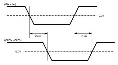
Figure 6. LVDS Output Propagation Delay
