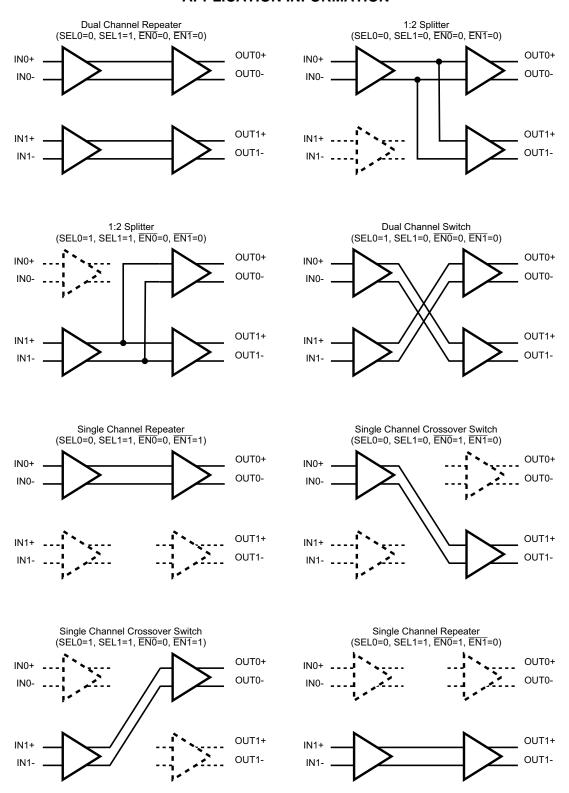
Figure 3. DS90CP02 Configuration Select Decode
