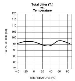
Total Jitter measured at 0V differential while running a PRBS  $2^{23}$ -1 pattern in dual channel repeater mode.  $V_{CC} = 3.3V, V_{ID} = 0.5V, V_{CM} = 1.2V, 1.5$  Gbps data rate Figure 9.
