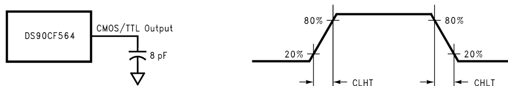
Figure 6. DS90CF564 (Receiver) CMOS/TTL Output Load and Transition Times
