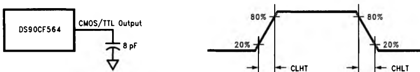
FIGURE 4. DS90CF564 (Receiver) CMOS/TTL Output Load and Transition Times
