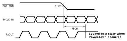
Figure 21. Receiver Powerdown Delay
