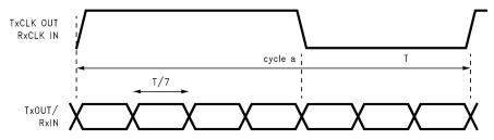
Figure 18. Seven Bits of LVDS in One Clock Cycle
