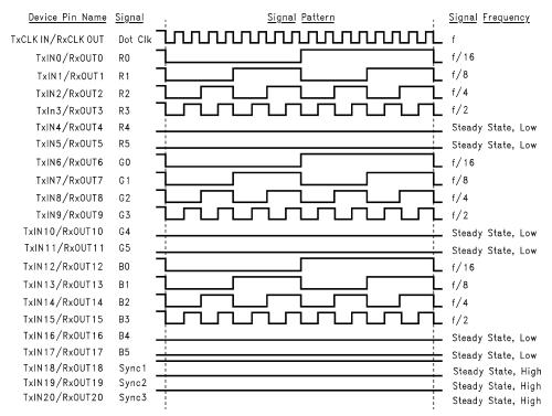
The worst case test pattern produces a maximum toggling of device digital circuitry, LVDS I/O and TTL I/O.
