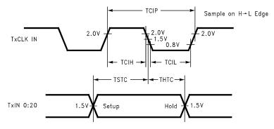
Figure 12. DS90CF561 (Transmitter) Setup/Hold and High/Low Times
