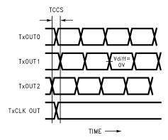
Measurements at Vdiff = 0V
