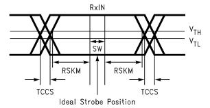
SW—Setup and Hold Time (Internal Data Sampling Window)
