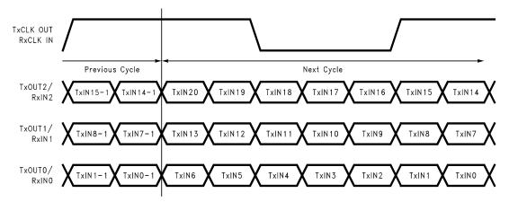
Figure 19. 21 Parallel TTL Data Inputs Mapped to LVDS Outputs (DS90CF561)
