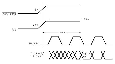
Figure 16. DS90CF561 (Transmitter) Phase Lock Loop Set Time
