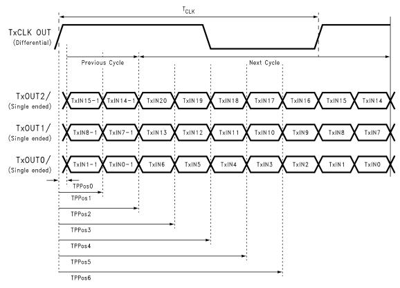
Figure 22. Transmitter LVDS Output Pulse Position Measurement
