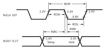
Figure 13. DS90CF562 (Receiver) Setup/Hold and High/Low Times
