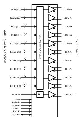
Figure 1. Transmitter Block Diagram
