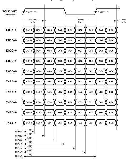
Figure 15. LVDS Input Mapping and Ideal Transmitter Pulse Position
