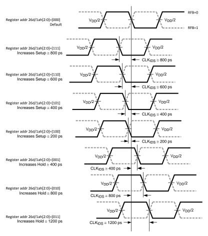
Figure 14. User Programmable Internal Clock Delay Adjustment for Input Data Setup/Hold Optimization Input Data Sampling Clock (TCLK<sub>IDS</sub>)
