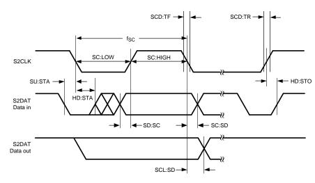
Figure 3. Two-Wire Serial Communication Interface Timing Diagram
