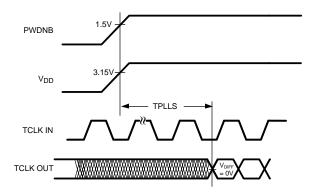
Figure 10. Phase Lock Loop Set Time
