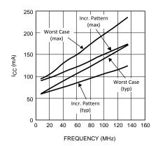
Figure 6. Typical and Max ICC with Worst Case and Incremental Test Pattern
