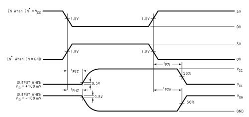
Figure 7. Receiver TRI-STATE Delay Waveforms
