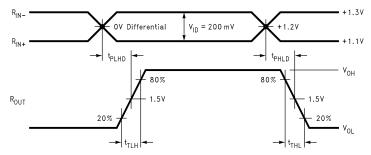
Figure 5. Receiver Propagation Delay and Transition Time Waveforms
