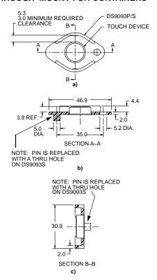
The DS9093S and DS9093P allows the user to permanently attach a Touch Memory to an object with one or two screws, rivets, etc. The plastic plate is designed with an inset that accommodates the flange of the F5
