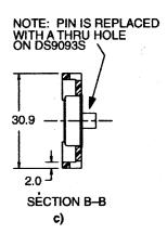
The DS9093S and DS9093P allow the user to permanently attach an <u>i</u>Button to an object with one or two screws, rivets, etc. The plastic plate is designed with an inset that accommodates the flange of the F5 package and allows for flush mounting. A protective wall is provided along the sides of the plate to reduce incidental damage to the <u>i</u>Button.
