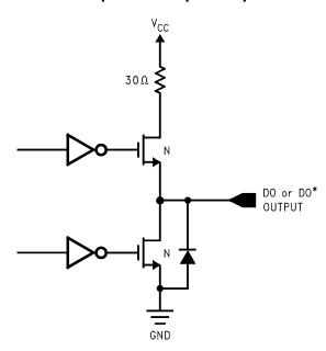
Figure 16. Driver Output Equivalent Circuit
