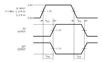
Figure 4. Propagation Delays
