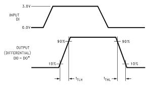
Input pulse; f = 1 MHz, 50%,  $t_r \le 6$  ns,  $t_f \le 6$  ns
