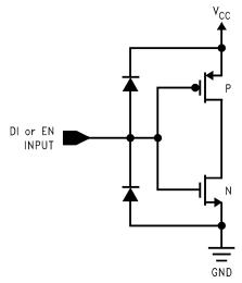
Figure 17. Driver Input or Driver Enable Equivalent Circuit
