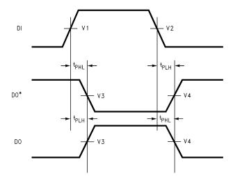
Figure 15. Waveforms for Circuit 4 – Waveforms for Circuit 4 (See Figure 14)
