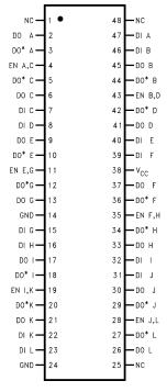
Figure 1. 48-Pin SSOP Package See Package Number DL0048A
