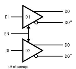
Figure 2. Functional Diagram
