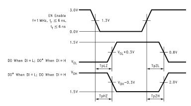
Figure 5. Enable and Disable Times
