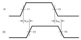
Figure 10. Waveforms for Circuit 1 – Propagation Delay Waveforms for Circuit 1 and Circuit 2 (See Figure 9)
