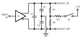
C1 = C2 = C3 = 40 pF (including Probe and Jig Capacitance), R1 = R2 =  $50\Omega$ , R3 =  $500\Omega$
