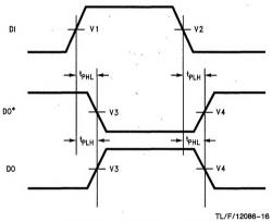
FIGURE 11. Waveforms for Circuit 4 (See Figure 10)
