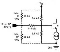
FIGURE 10. Receiver Input Equivalent Circuit
