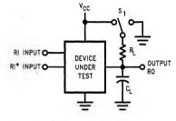
FIGURE 2. Test Circuit for Switching Characteristics
