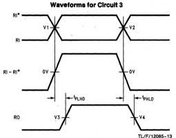
FIGURE 8. Propagation Delay Waveforms for Circuit 3 (see Figure 7)
